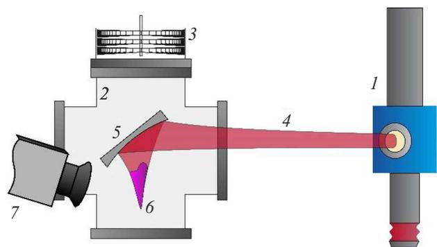
**Figure 1.** Schematic diagram of the experimental setup. 1 — gyrotron, 2 — vacuum discharge chamber, 3 — turbomolecular pump, 4 — THz-beam, 5 — focusing mirror, 6 — beam focus/discharge, 7 — Nanogate-24 chamber.
