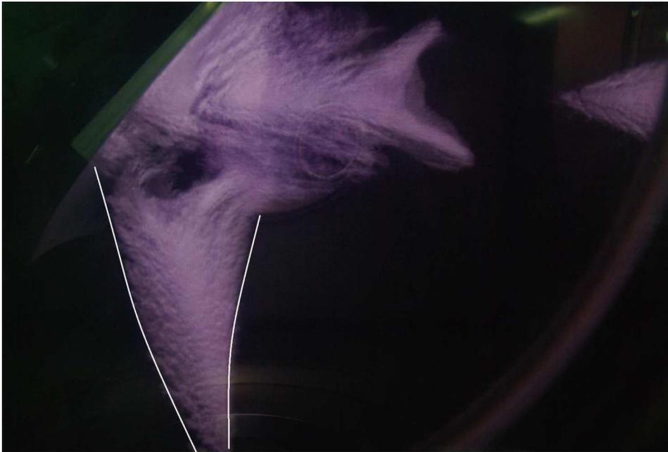
**Figure 2.** Photograph of the discharge in argon. Heating radiation frequency 250 GHz, gas pressure 50 Torr. The electromagnetic radiation propagates from right to left to the focusing mirror and then from top to bottom. Light lines schematically show the boundaries of the focused beam.
