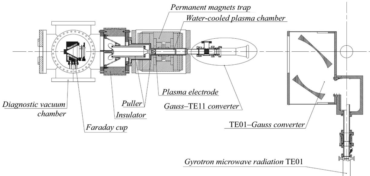
**Figure 2.** Schematic of the GISMO experimental setup (the microwave-radiation source is not shown).
