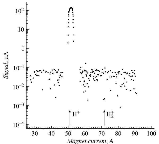
**Figure 3.** Composition of the extracted ion beam at a heating power of 5 kW and pressure in the discharge chamber  $2 \cdot 10^{-3}$  Torr (dependence of the beam current passed through the magnetic analyzer on the magnet current).
