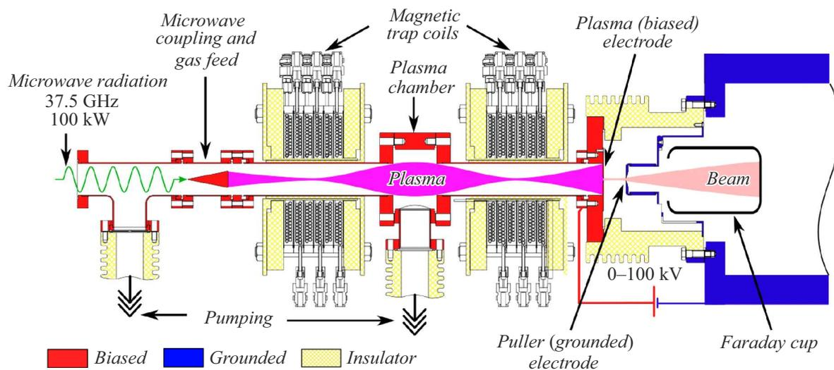
**Figure 1.** Schematic of the SMIS experimental setup (the microwave radiation source is not shown). A color version of the figure is provided in the online version of the paper.
