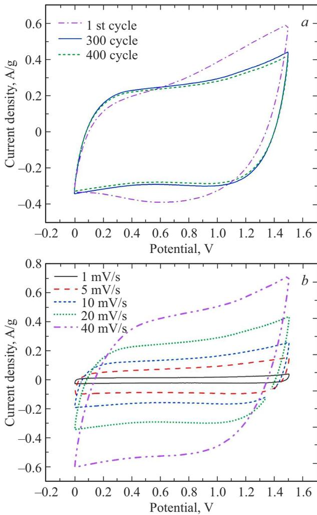
**Figure 2.** *a* — CV curves of asymmetric supercapacitor cell at the initial stages of measurements (potential sweep rate 5 mV/s); *b* — family of CV curves measured at different potential scan rates.
