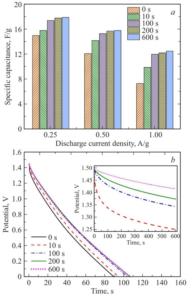
**Figure 3.** Characteristics of an asymmetric SC vs. the time of additional charge in potentiostatic mode at maximum voltage (1.5 V): *a* — specific capacitance at different current densities; *b* — discharge curves measured at charge/discharge current density of 0.25 A/g (the insert shows the self-discharge curves of asymmetric SC).
