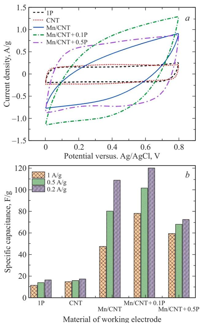
**Figure 1.** *a* — CV characteristics of the electrodes measured at scan rate of 10 mV/s; *b* — specific capacitance of electrodes at different values of discharge current density.
