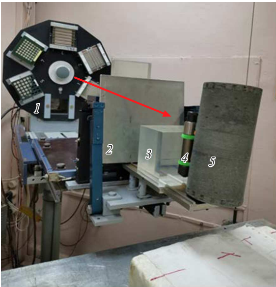
Figure 2. Polymer composite irradiation set up using a synchrotron (red arrow shows the proton beam outgoing direction from the synchrotron channel), where: 1 — synchrotron, 2 — 4 mm aluminum shutter, 3 — water absorber (was not used for this experiment), 4 — „PILLE-MKS“ sensor and passive TLD and STD assembly, 5 — polymer composite.
