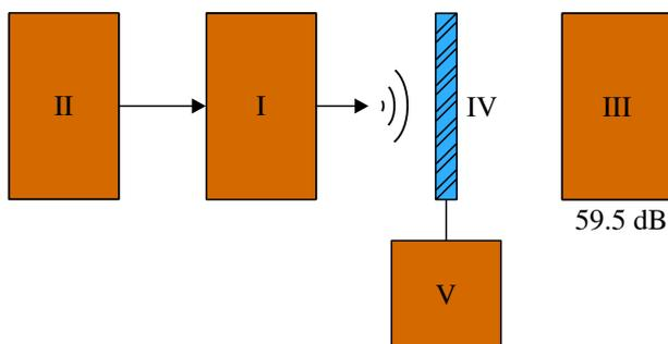
**Figure 3.** The design of the experiment № 3 to determine the pressure level on the sound meter III at a fixed distance between the sound meter and the speaker I and a fixed level of the speaker radiation. Matrix III is located between the speaker and the sound level meter in the pump mode.
