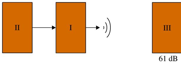
**Figure 1.** Scheme of the experiment № 1 to determine the pressure level on the sound meter III at a fixed distance between the sound meter and the speaker I and a fixed level of the speaker radiation. There are no obstacles between the speaker and the noise meter.
