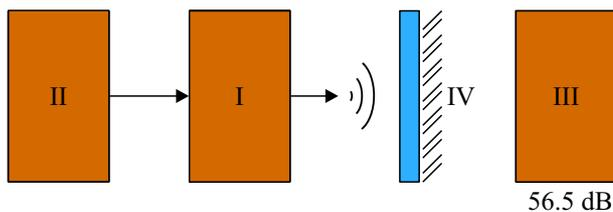
**Figure 2.** The design of the experiment № 2 for determining the level of pressure on the sound meter III with a fixed distance between the sound meter and the speaker I and a fixed level of the speaker radiation. Matrix III is located between the speaker and the noise meter in the non-pumping mode.
