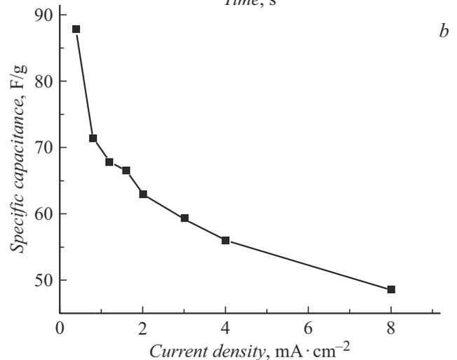
**Figure 3.** Charge-discharge curves (a) and specific capacitance (b) of an electrochemical cell at different current densities.
