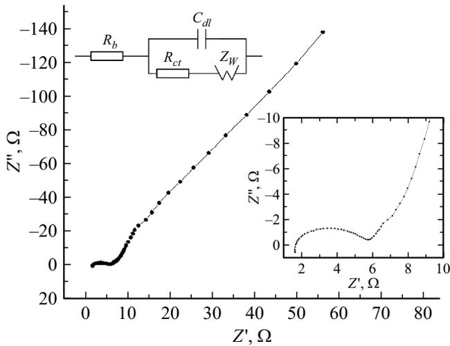
**Figure 1.** Impedance locus of an electrochemical cell. The upper inset shows — equivalent scheme (high frequency region of the locus).
