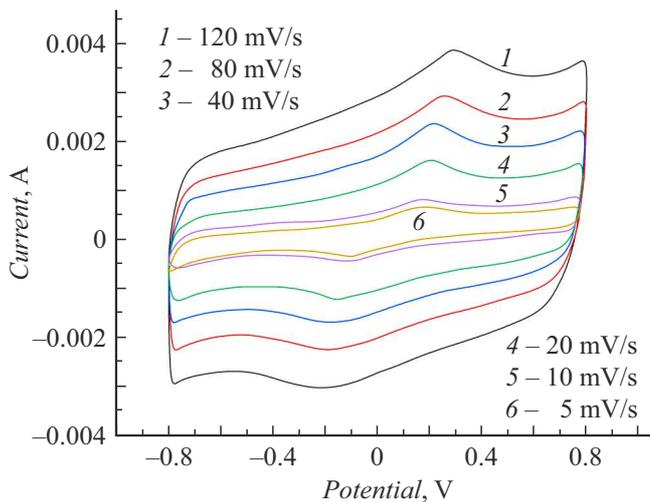
**Figure 2.** Cyclic voltammogram of an electrochemical cell at different potential sweep rates.
