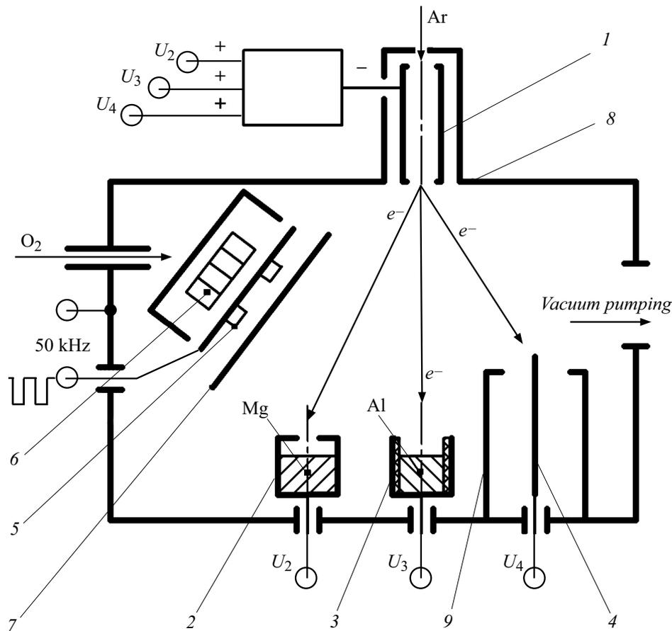
**Figure 1.** Schematic diagram of thin film deposition setup  $\text{MgAl}_2\text{O}_4$ : self-pumped cathode (1), crucibles (2, 3), rod-type anode (4), samples (5), heater (6), shutter (7), vacuum chamber (8), screen (9).
