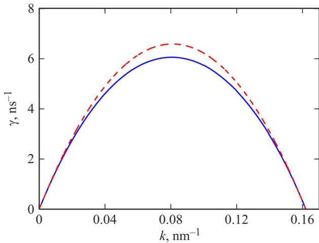
**Figure 2.** Dependence of the EHD-instability increment  $\gamma$  on the wave number  $k$  for the exact dispersion law (solid line) and the parabolic approximation (dashed line). Field  $E = E_v/2 \approx 4.9 \cdot 10^7$  V/cm; liquid copper at melting point.
