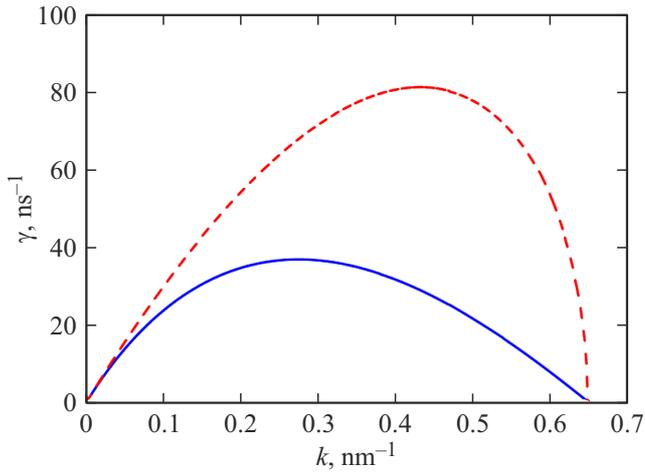
**Figure 1.** Dependence of the EHD-instability increment  $\gamma$  on the wave number  $k$  with (solid line) and without (dashed line) viscous effects. Field  $E = E_v \approx 9.8 \cdot 10^7$  V/cm; liquid copper at melting point.
