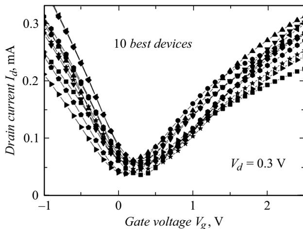
**Figure 3.** The characteristics of the best ten (out of about 50) devices demonstrating their relatively low spread.
