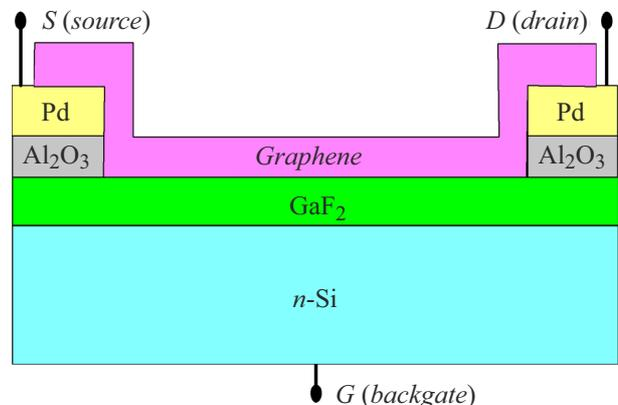
**Figure 1.** The structure of the studied field-effect transistor. The graphene film serves as a current-conducting layer, and fluoride — as a gate insulator (earlier, other combinations of materials were used in such devices:  $\text{MoS}_2/h\text{BN}/\text{Si}$ , etc.).
