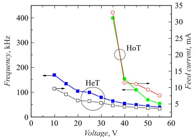
**Figure 1.** Dependences of the maximum frequency of generation of current pulses in the thyristor–capacitor circuit, as well as the average supply current on the blocking voltage for thyristors based on HoT and HeT structures. The capacitance of the capacitor is 1 nF.
