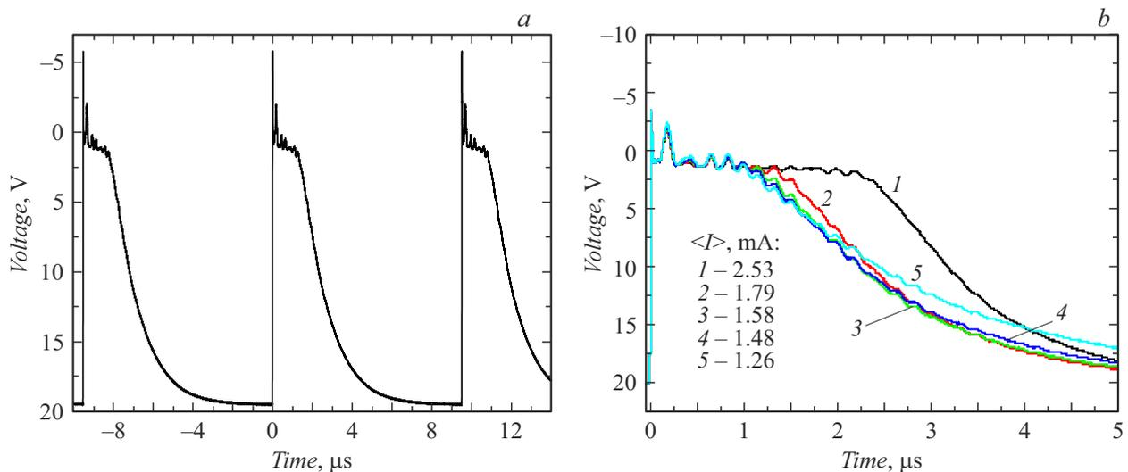
**Figure 3.** *a* — The time dependence of capacitor voltage in the maximum repetition rate mode. *b* — time dependence of the capacitor voltage for different average power supply currents  $\langle I \rangle$ . Blocking voltage is 20 V, thyristor key based on HeT structure, capacitor capacitance is 1 nF.
