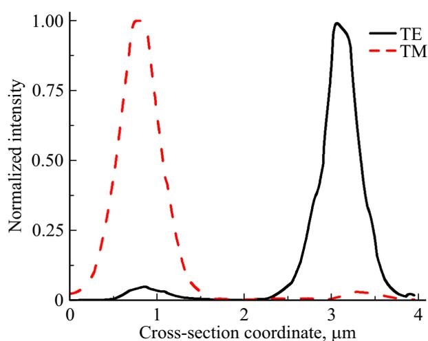
**Figure 3.** Normalized intensity distribution at the output of the PS for TE and TM modes.
