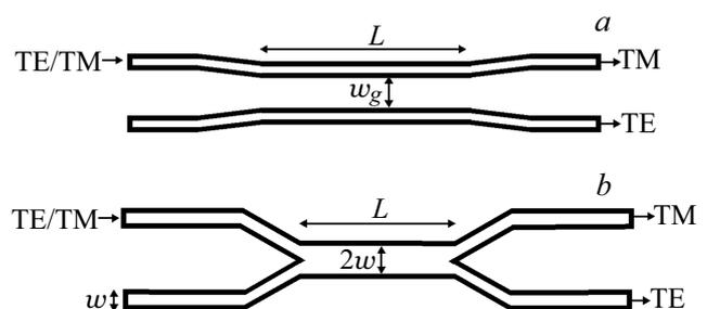
**Figure 1.** Typical PS configurations are: *a* — PS based on a conventional directional coupler, *b* — PS based on zero gap directional coupler.
