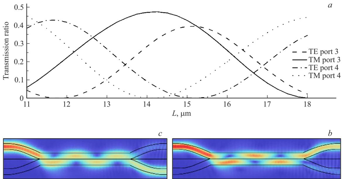
**Figure 2.** Results of numerical simulation: *a* — dependence of the port transmittance coefficient on the type of mode and the length of the two-mode interference zone, *b* — calculation of the propagation of the TE mode for the length of the two-mode interference zone  $14.5 \mu\text{m}$ , *c* — calculation of the propagation of the TM mode with a two-mode interference zone length of  $14.5 \mu\text{m}$ .
