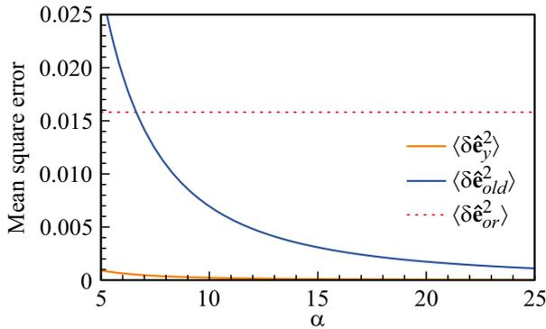
**Figure 6.** Mean square error  $y$ -quadrature of the teleported state depending on the displacement of the non-Gaussian resource  $\alpha$ : orange — for the protocol with the phase correction, blue — for the protocol without the phase correction when teleporting the vacuum state. The red dotted line indicates the level of teleportation error in the original scheme. The squeezing level of resource oscillators is  $-15$  dB.
