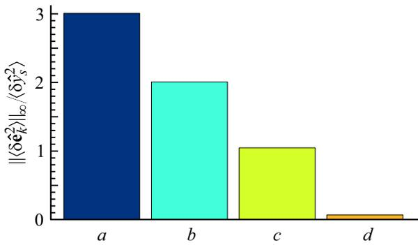
**Figure 4.** Error in various implementations of the CZ transformation: *a* — on an unweighted four-node linear cluster, *b* — on a pair of two-node clusters, *c* — on a weighted four-node linear cluster, *d* — with a cubic phase gate.
