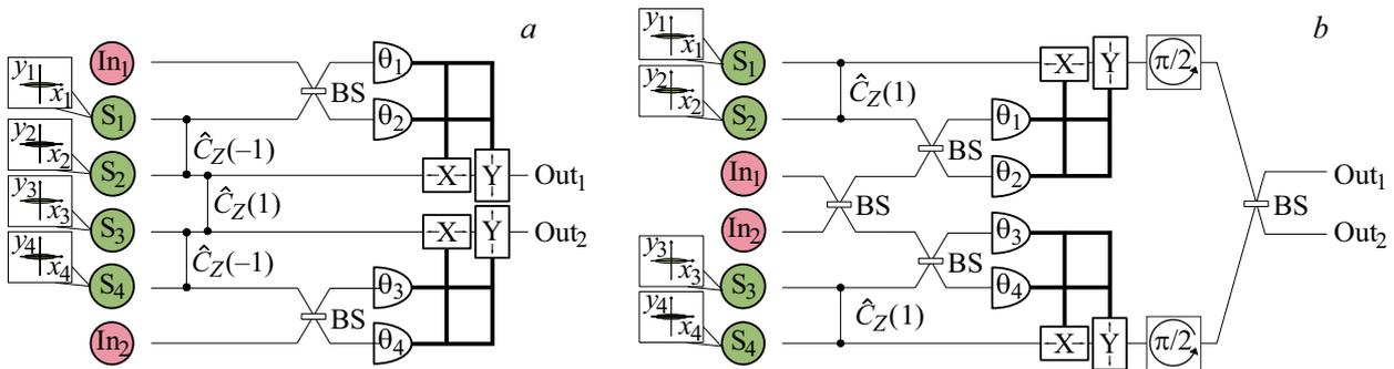
**Figure 3.** (a) Scheme of the implementation of the CZ transformation on a unweighted four-node linear cluster. (b) Scheme of the implementation of the CZ transformation on a pair of two-node clusters. BS — a symmetrical beamsplitter.
