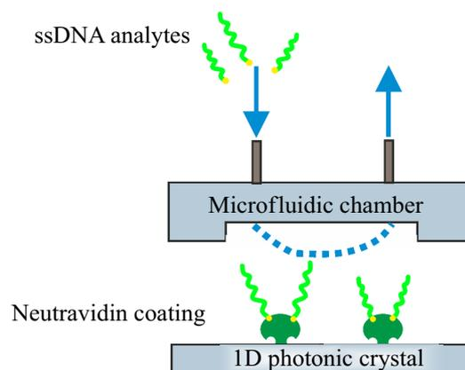
**Figure 1.** Schematics of the detection of model single-stranded DNAs in a flow using a microfluidic platform and a sensor based on a one-dimensional photonic crystal. The arrows indicate the directions of injection and removal of the analyte from the microfluidic platform. Designations: ssDNA, single-stranded DNA; 1D, one-dimensional.
