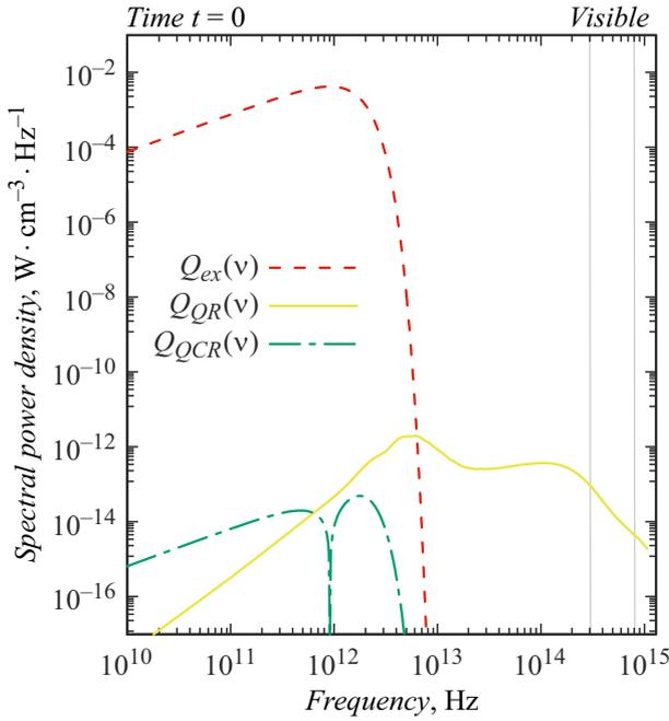
**Figure 5.** Spectral power densities of radiation with  $E_0 = 250 \text{ kV/cm}$ ,  $\tau = 2.46 \cdot 10^{-13} \text{ c}$ .
