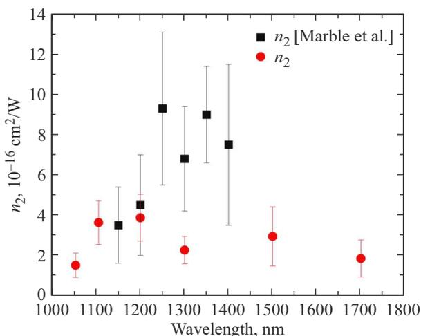
**Figure 4.** Nonlinear refraction indices of water (red dots) calculated using equation (1). Comparison of the data with findings of [16,17] (black dots).
