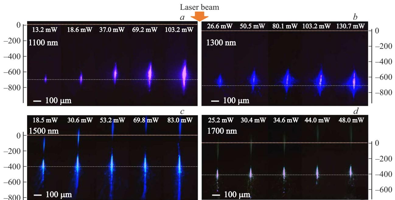
**Figure 2.** Plasma channel images in distilled water for 1100 nm (a), 1300 nm (b), 1500 nm (c) and 1700 nm (d) and various mean powers of laser pumping emission that are shown in the figure. Orange lines correspond to the cell water surface, white dashed line shows the focal plane position. Depth scales in  $\mu\text{m}$  are shown on the right and left of the pictures.
