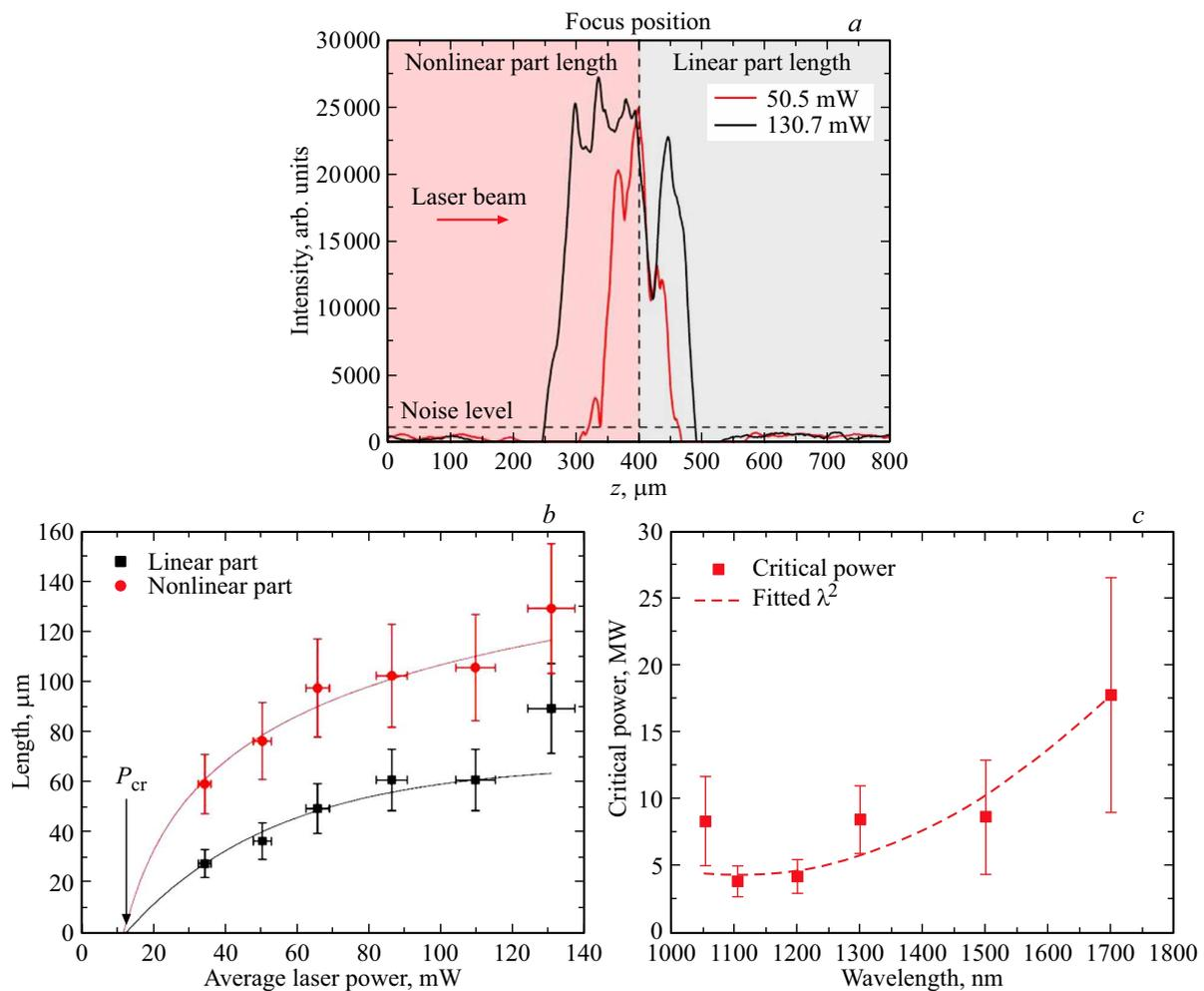
**Figure 3.** (a) Example of identifying „linear“ and „nonlinear“ plasma channel length for 1300 nm and a mean power of 50.5 mW and 130.7 mW by the luminous intensity profiles of the channel on the  $z$  axis; (b) „linear“ and „nonlinear“ plasma channel lengths for 1300 nm pumping; (c) dependence of the critical self-focusing power  $P_{cr}$  on the pumping wavelength (red dots) and its approximation by function quadratic in wavelength (red dashed line).
