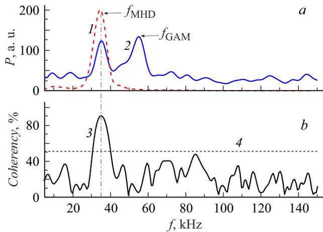
**Figure 1.** *a* — Power spectra for signals of the MHD probe (1) and  $f_D(t)$  (2); *b* — coherence spectrum for these signals (3) and noise coherence level (4).
