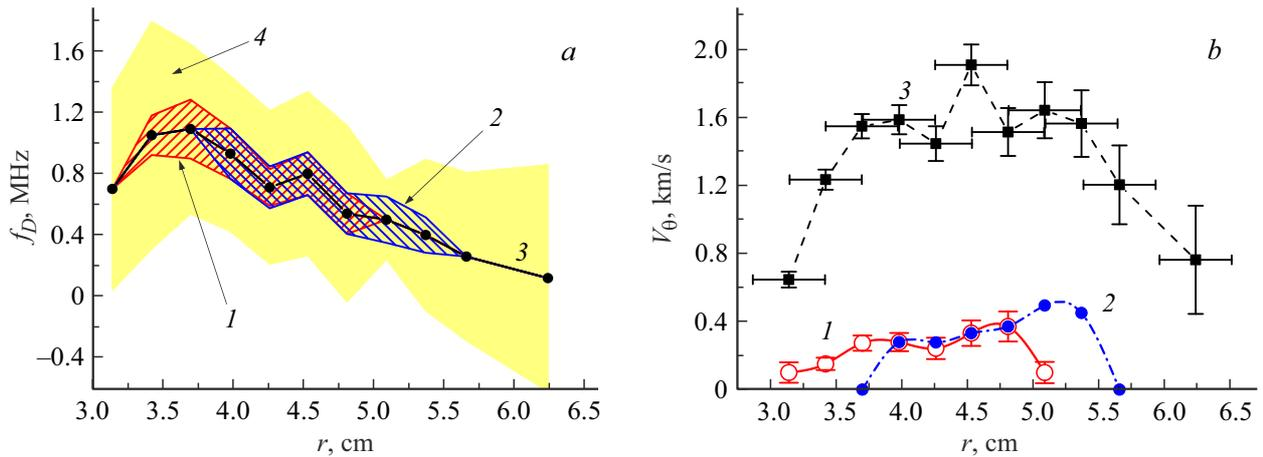
**Figure 2.** *a* — Radial profiles of parameters characterizing Doppler frequency shift  $f_D(t)$ : amplitudes of its oscillations at MHD (1) and GAM (2) frequencies relative to the mean level (3) against the background of its dispersion (4); *b* — radial profiles of parameters characterizing velocity  $V_\theta$ : amplitudes of its oscillations at MHD (1) and GAM (2) frequencies and the mean value (3).
