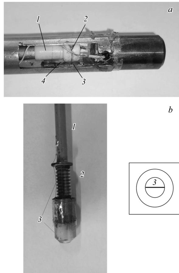
**Figure 1.** *a)* Image of the near-field microwave probe for scanning along the film: 1 — coaxial cable, 2 — wire of the near-field microwave probe, 3 — HTSC film, 4 — Teflon film; *b)* image of a near-field microwave probe for measuring the anisotropy of nonlinear microwave properties of superconductors: 1 — coaxial cable, 2 — spring, 3 — wire of a near-field microwave probe. The insert for the case (b) shows the bottom view.
