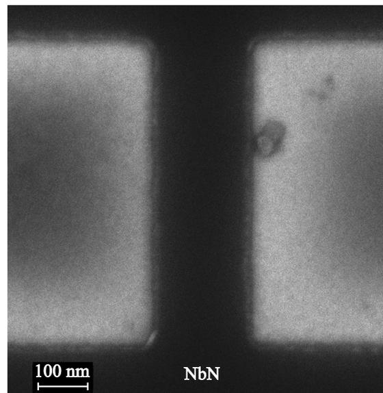
**Figure 2.** SEM image of a NbN nanowire (dark region) with a thickness of 5 nm, a width of 200 nm and a length of 600 nm on a substrate of single-crystal sapphire.
