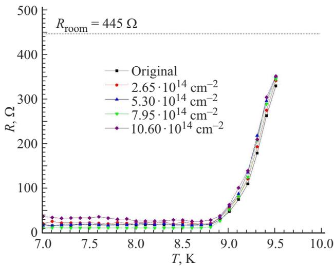
**Figure 5.** The dependences of the electrical resistance of  $20\ \mu\text{m}$  wide samples on the temperature at various fluences of ion irradiation, based on the current-voltage curve.
