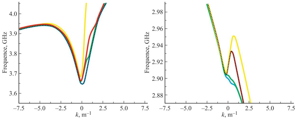
**Figure 2.** The dispersion characteristics for a structure with a metal shield near the layer with the lowest magnetization at various parameters of the electrical conductivity of the metal shield: 59980000 S/m (yellow line), 90000 S/m (red line), 37500 S/m (green line), 3750 S/m (blue line) and the dispersion characteristics obtained as a result of solving the analytical equation (black dotted curve).
