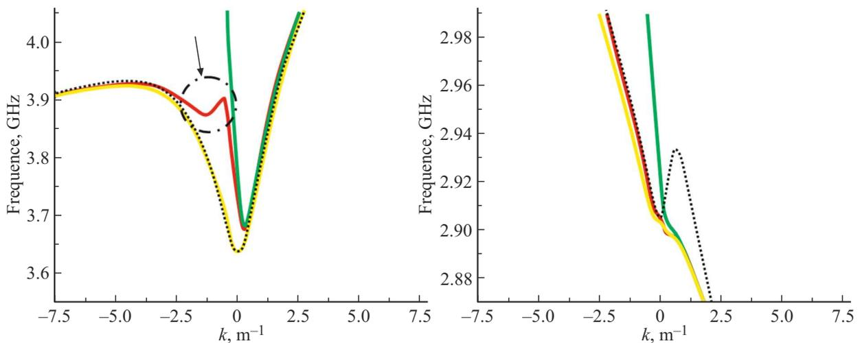
**Figure 3.** Dispersion characteristics for a structure with a metal shield near the layer with the highest magnetization at various parameters of the electrical conductivity of the metal shield: 59980000 S/m (yellow line), 90000 S/m (red line), 3750 S/m (green line) and the dispersion characteristics obtained as a result of solving the analytical equation (black dotted curve).
