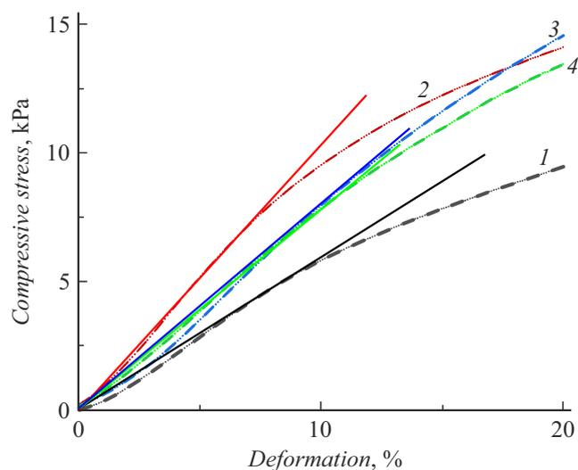
Typical deformation curves of synthesized PIF samples (BZP–DADPM) with different MMT contents. 1 — sample free of MMT, 2 — sample with 0.5 mass% of MMT, 3 — sample with 1 mass% of MMT, 4 — sample with 3 mass% of MMT.
