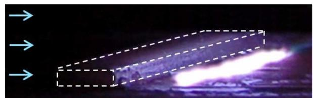
**Figure 4.** Integral shot of discharge plasma optical glow in flow downstream SW. Arrows indicate flow direction, dashed line — obstacle boundaries.
