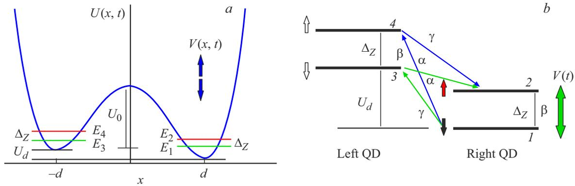
**Figure 1.** *a* — scheme of the lower four levels  $E_1$ – $E_4$  in a double quantum dot with potential  $U(x, t)$  (blue curve) for the Hamiltonian (1). *b* — transitions between levels 1, 2 in the right QD and 3, 4 in the left QD with matrix elements  $\alpha$ ,  $\beta$ ,  $\gamma$  for the Hamiltonian matrix notation (3). (A color version of the figure is provided in the online version of the paper).
