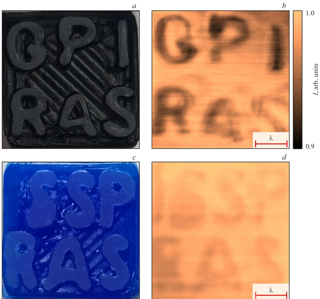
Figure 5. Terahertz SI microscopy of objects with subwavelength-scale inhomogeneities. (a)–(d) Photographic and THz images of 3D-printed polymer logos of the Prokhorov General Physics Institute (GPI RAS; the logo is made of conductive ABS) and the Osipyan Institute of Solid State Physics (ISSP RAS; PLA polymer).
