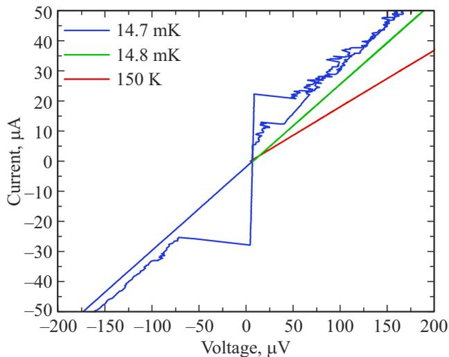
**Figure 5.** Current-voltage curves for H1030 structure at temperatures of 150, 14.8 and 14.7 mK.
