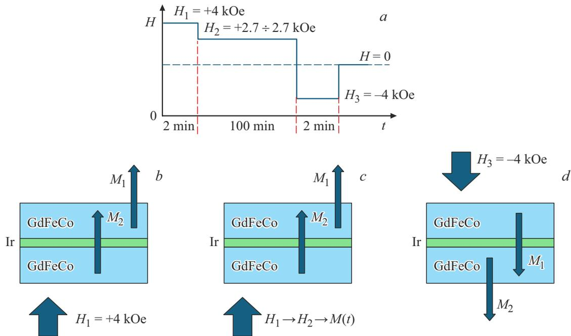
**Figure 1.** Field switching diagram in single cycle of experiment on preparation of time dependences of magnetic moment (a). Sample saturation in field  $H_1 = +4\text{ kOe}$  (b). Field switching from  $H_1$  to  $H_2$  in range from  $+2.7$  to  $-2.7\text{ kOe}$ , and recording of time dependence of magnetic moment (c). Sample saturation in reverse field  $H_3 = -4\text{ kOe}$  (d). The external magnetic field was then reduced to zero before the start of the next cycle.
