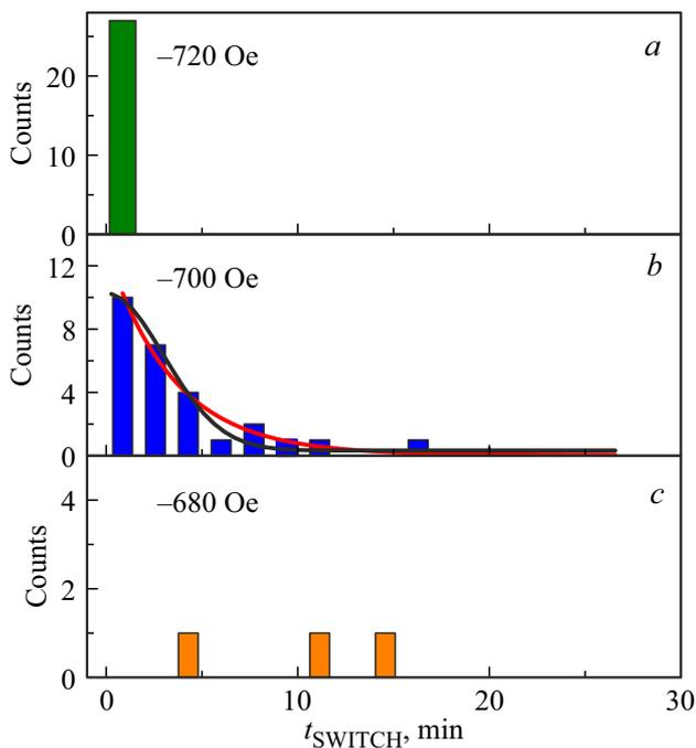
**Figure 6.** Distributions of probability of switching from state  $AP^+$  to  $AP^-$  by delay time  $t_{\text{SWITCH}}$ , obtained in fields  $H_2 = -720$ ,  $-700$  and  $-680$  Oe. Figure 6, *b* by lines shows approximation by normal (green line) and exponential (red line) distributions. For normal distribution average time of event is  $\sim 3$  min, and for exponential  $\sim 4$  min.
