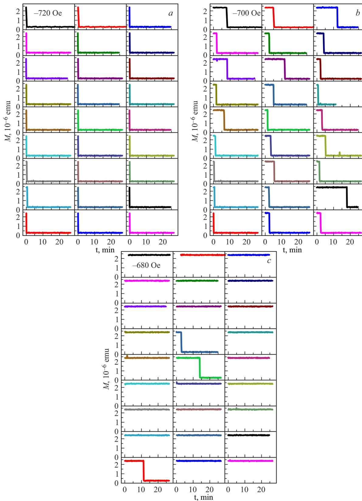
**Figure 5.** Set of time dependence of magnetic moment at  $H_2 = -720$  Oe (*a*), 700 Oe (*b*) and  $-680$  Oe (*c*) for transition  $AP^+ \rightarrow AP^-$ .
