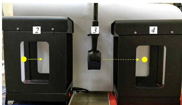
Figure 3. Experimental test bench: 1 — pneumatic TB accelerator (not shown in the figure); 2 — chronograph-1 for determining the input speed; 3 — sample holder; 4 — Chronograph-2 for determining the output speed; 5 — TB absorber (not shown in the picture).
