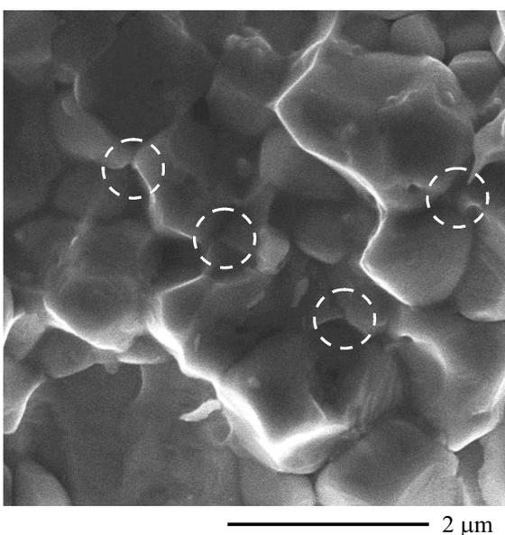
**Figure 6.** Electronic image of ceramics synthesized using modified two-stage technique. Typical triple points of grain boundaries contact are marked by dashed circles.
