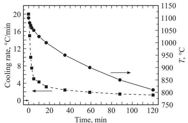
**Figure 2.** Temperature change from  $T_1$  to  $T_2$  without forced cooling.
