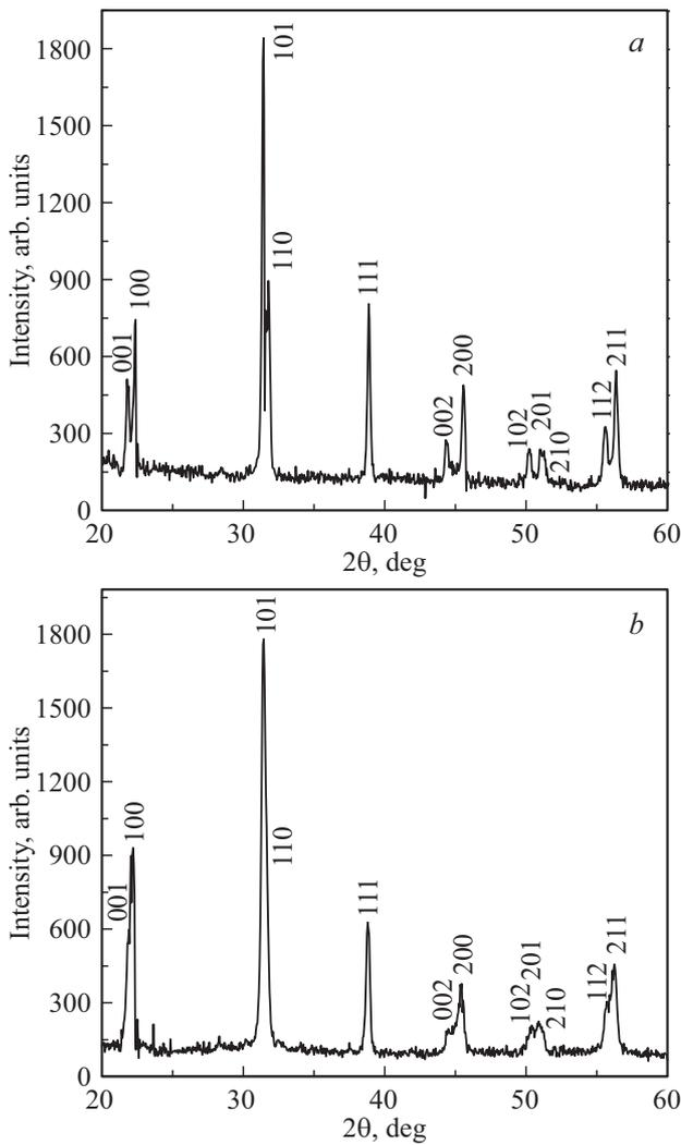
**Figure 3.** X-ray patterns of samples obtained using single-stage (*a*) and modified (*b*) two-stage sintering.
