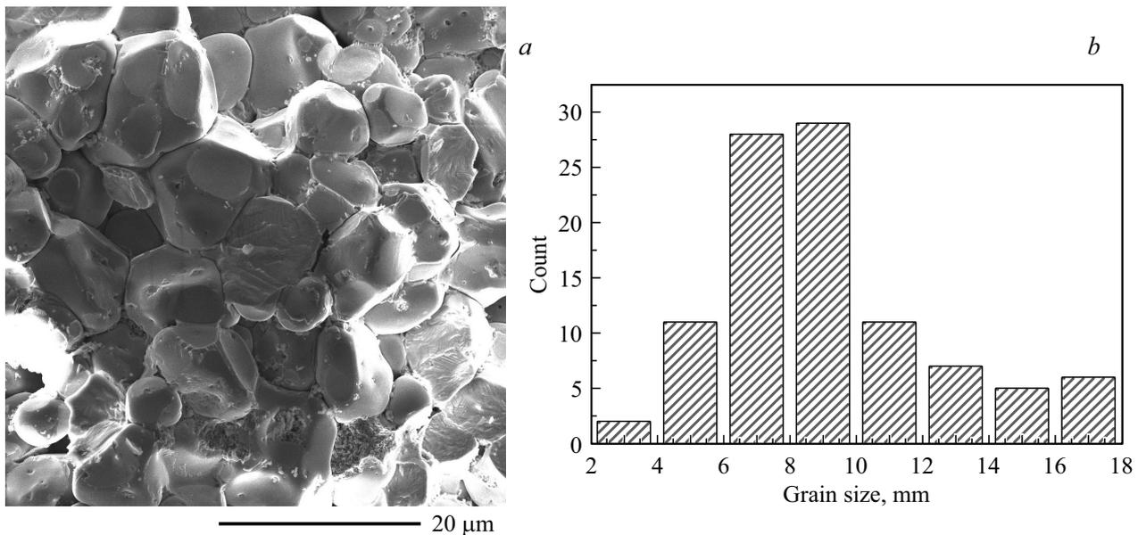
**Figure 5.** *a* — electronic image of end face of ceramics, obtained as result of single-stage firing, and *b* — grain size distribution histogram.
