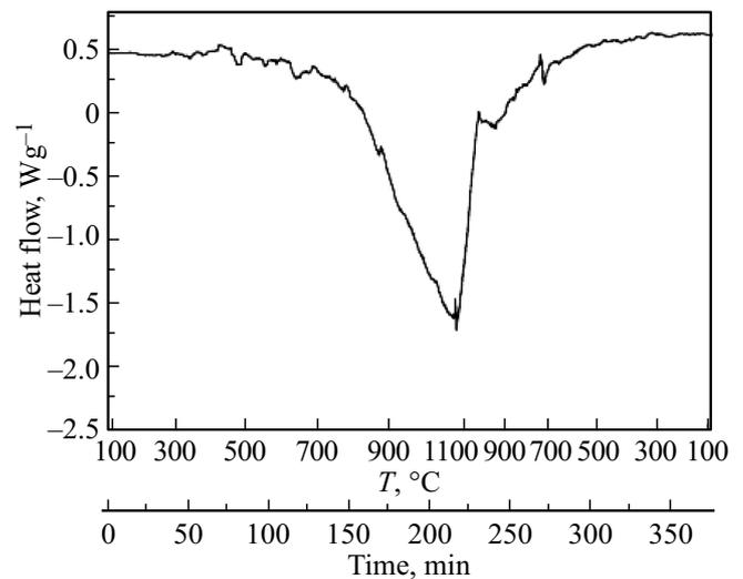
**Figure 1.** Results of differential thermal analysis obtained during reproduction of the temperature and time modes of modified sintering of BSPT.
