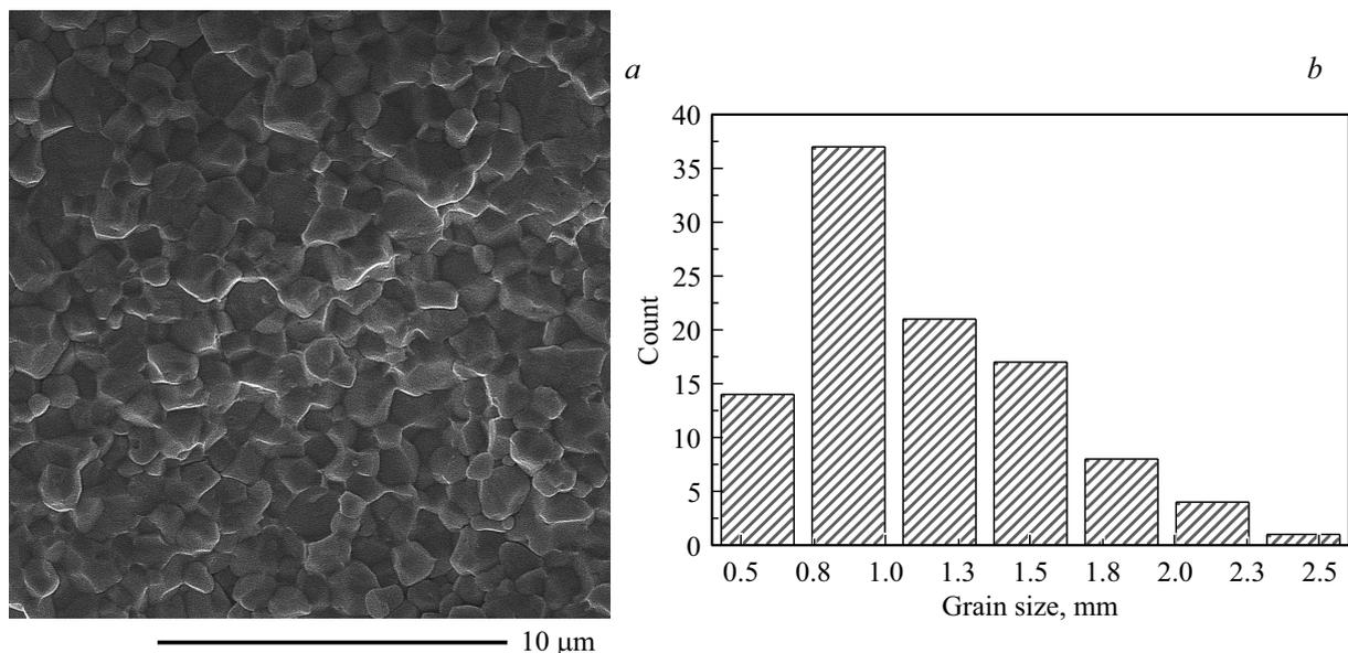
**Figure 4.** *a* — Electronic image of end face of ceramics, obtained as result of modified two-stage sintering, and *b* — grain size distribution histogram.
