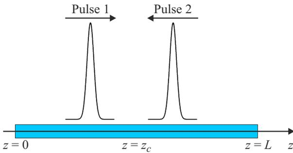
A pair of half-cycle pulses moves over the medium from opposite directions and collides in the center of the medium in a point with coordinate  $z = z_c$ .
