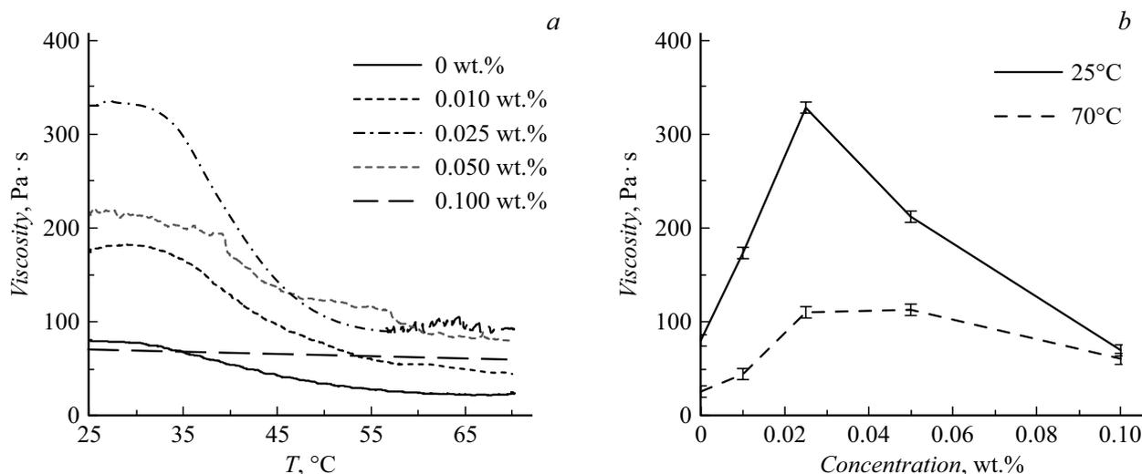
**Figure 1.** Effective viscosity of SWCNTmodified gels versus temperature (a) and concentration (b).
