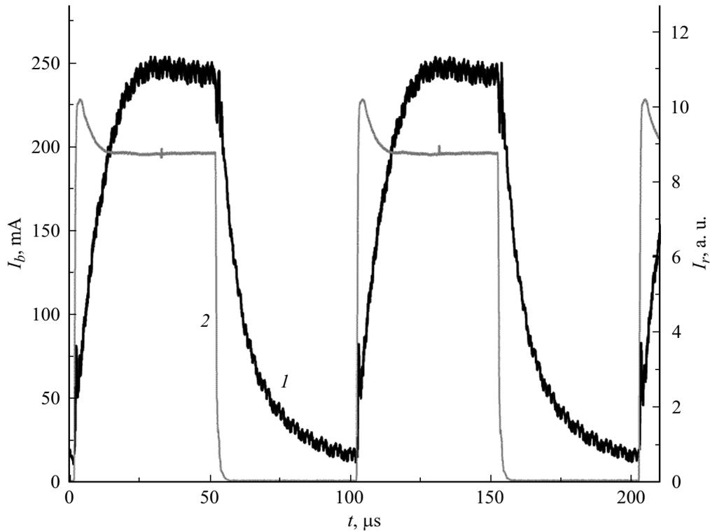
**Figure 1.** Time dependence of extracted ion current  $I_b$  (1) and amplitude of the RF current through the antenna  $I_r$  (2). The working gas (argon) flow rate is 24 sccm, RF power is 140 W, pulsation frequency is 10 kHz, no external magnetic field.
