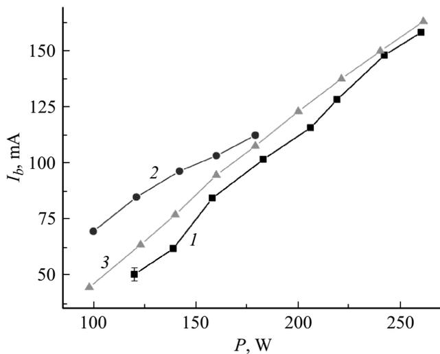
**Figure 2.** Extracted ion current  $I_b$  versus time-average RF power for the continuous mode (1) and pulse modes with duty factors of 40 (2) and 70% (3). The working gas (nitrogen) flow rate is 24 sccm, external magnetic field induction is 19 G, pulsation frequency is 10 kHz.
