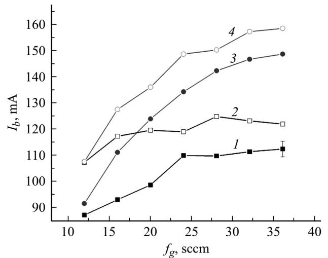
**Figure 3.** Extracted ion current  $I_b$  versus working gas flow rate for nitrogen (1, 2) and oxygen (3, 4). Curves 1 and 3 correspond to the continuous operating mode, while curves 2 and 4 are for the pulse mode with the pulsation frequency of 10 kHz and duty factor of 70%. RF power is 200 W, external magnetic field induction is 19 G.
