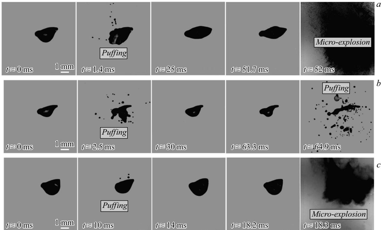
**Figure 2.** Video frames of two-liquid droplet fragmentation in the puffing and microexplosion modes ( $R_{d0} = 0.90 \pm 0.05$  mm,  $T_a = 750 \pm 10$  K). *a* — diesel fuel 90 vol.%, water 10 vol.%; *b* — kerosene 90 vol.%, water 10 vol.%; *c* — rapeseed oil 90 vol.%, water 10 vol.%.
