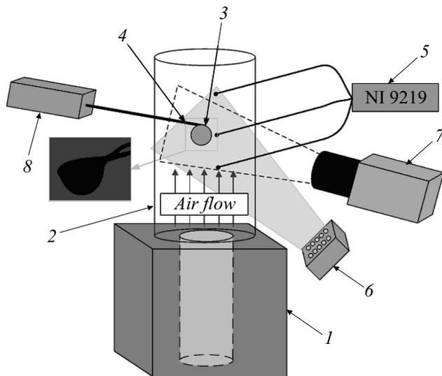
**Figure 1.** A test bench for measuring fragmentation characteristics of two-liquid droplets. 1 — tubular muffle furnace, 2 — thermally insulated cylinder, 3 — two-liquid droplet, 4 — holder, 5 — temperature recording system (National Instruments), 6 — light source, 7 — high-speed video camera, 8 — coordinate mechanism.
