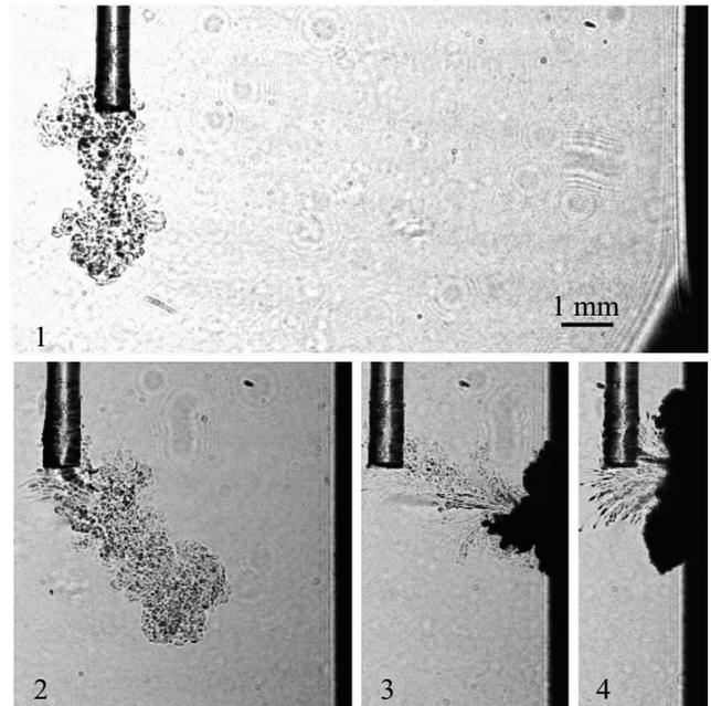
**Figure 2.** Response of a submerged jet to a flat solid surface as a function of  $\gamma$ :  $\gamma_1 = 3$  (frame 1),  $\gamma_2 = 1.26$  (frame 2),  $\gamma_3 = 0.77$  (frame 3), and  $\gamma_4 = 0.3$  (frame 4). The laser radiation power is  $P = 8 \text{ W}$ .
