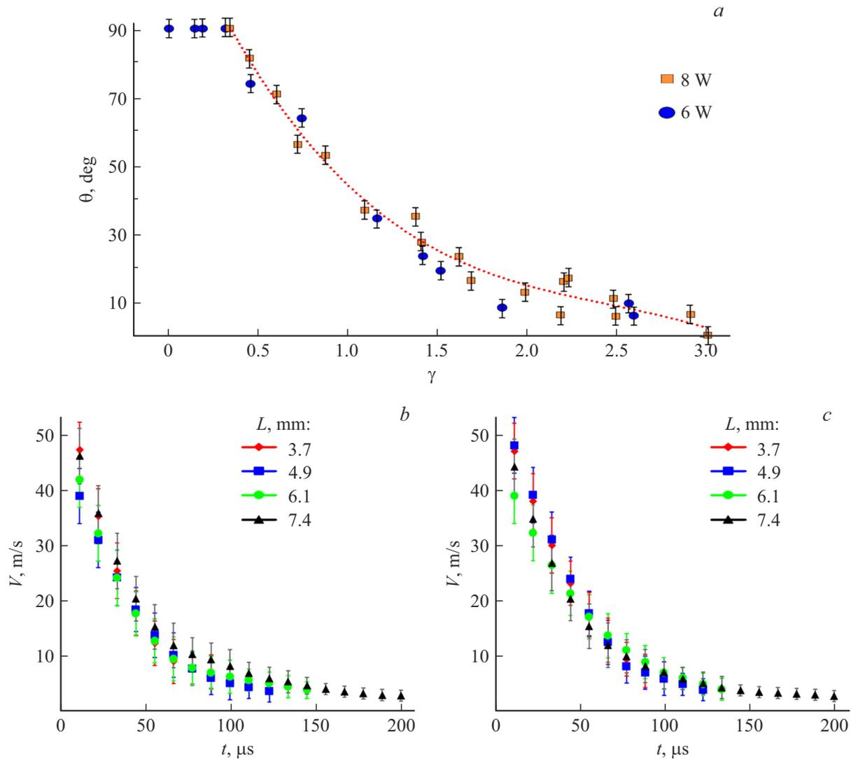
**Figure 3.** *a* — Dependence of the jet rotation angle on dimensionless distance  $\gamma$ . The dotted line represents the approximation of measurements by a third-degree polynomial. *b* and *c* — Time dependences of the submerged jet front velocity at different distances  $L$  and laser radiation powers of 6 (*b*) and 8 W (*c*).
