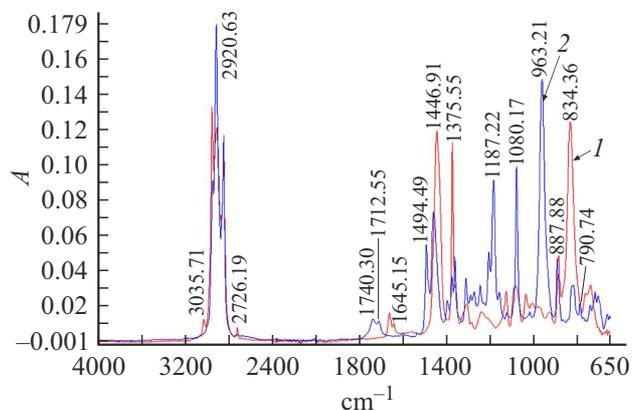
**Figure 5.** IR spectra of samples of rubber SKI-5 PM (*I* (red curve) — original rubber, 2 (blue curve) — dried rubber extract).
