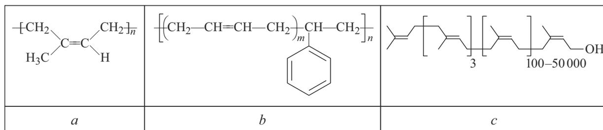
**Figure 1.** Structural formulas of the objects of research: *a* — structural formula of SKI-5 PM rubber (*cis*-1,4-isoprene); *b* — structural formula of SKMS-30 ARKM-27 rubber; *c* — the structural formula of NR.
