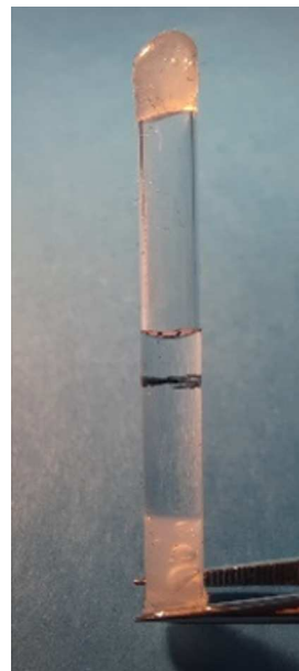
The gel sample is in a glass capillary sealed on both sides with polymer caps.
