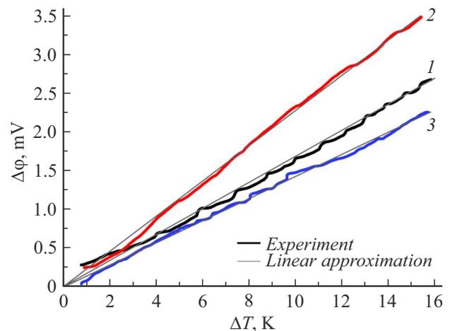
**Figure 3.** Dependence of the thermoelectric potential difference on the temperature difference for Ringer's solution samples with different potassium ion content. 1 — standard balance (4 mmol/L), 2 — excess ions (5.5 mmol/L), 3 — lack of ions (3 mmol/l). The temperature of the colder region is 18°C.
