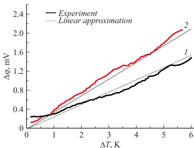
**Figure 4.** Dependence of the thermoelectric potential difference on the temperature difference for pig blood plasma samples with different potassium ion content. 1 — standard balance (7 mmol/l), 2 — excess ions (8 mmol/l). The temperature of the colder region is 18°C.
