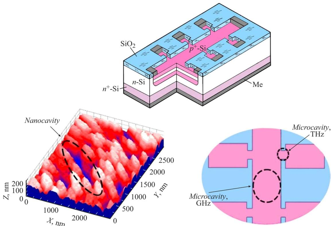
**Figure 1.** A silicon nanosandwich structure possessing nano- (on the surface of  $p^+$ -Si) and microresonators tuned to selected wavelengths of the spectral range, and used as an IR emitter with THz modulation. The image of the surface  $p^+$ -Si was obtained by scanning tunneling microscopy (STM).
