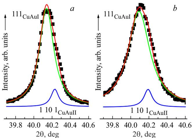
**Figure 8.** Sections of X-ray diffraction patterns near peaks  $(111)_{\text{CuAuI}}$  and  $(1101)_{\text{CuAuII}}$ , obtained from preliminary quenched (a) and deformed (b) samples of Cu-56Au alloy after annealing at temperature of  $300^{\circ}\text{C}$  for 1440 h. The experimental data are presented by dots, calculated data — by solid lines.
