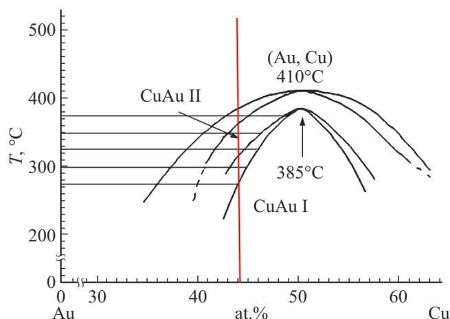
**Figure 1.** Section of equilibrium phase diagram of system Cu-Au from paper [11]. Vertical red line corresponds to composition of studied alloy Cu-56 at.% Au. Horizontal lines show temperatures at which experiments were performed: 275, 300, 325, 350 and 375°C.
