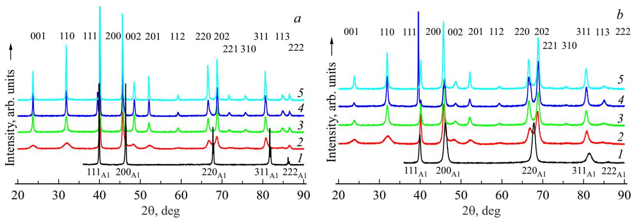
**Figure 2.** XRD results of samples of quenched (a) and deformed (b) alloy in initial state (1), after annealing for 1 (2), 24 (3), 168 (4) and 1440 h (5) at temperature of 275°C.
