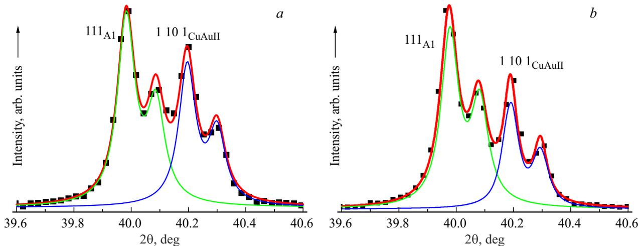
**Figure 7.** Sections of X-ray diffraction patterns with peaks  $(111)_{A1}$  and  $(110)_{1CuAuII}$  obtained from preliminary quenched (a) and deformed (b) samples of Cu-56Au alloy after annealing at temperature of  $375^{\circ}\text{C}$  for 1440 h. The experimental data are presented by dots, calculated data — by solid lines.
