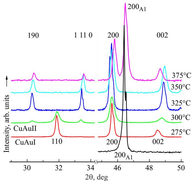
**Figure 6.** Sections of X-ray diffraction patterns in range of angles  $2\theta$  from 29° to 50°, obtained from preliminary quenched samples of Cu-56Au alloy annealed in temperature range from 275 to 375°C for 1440 h. In bottom for comparison the diffraction pattern of disordered alloy is shown.
