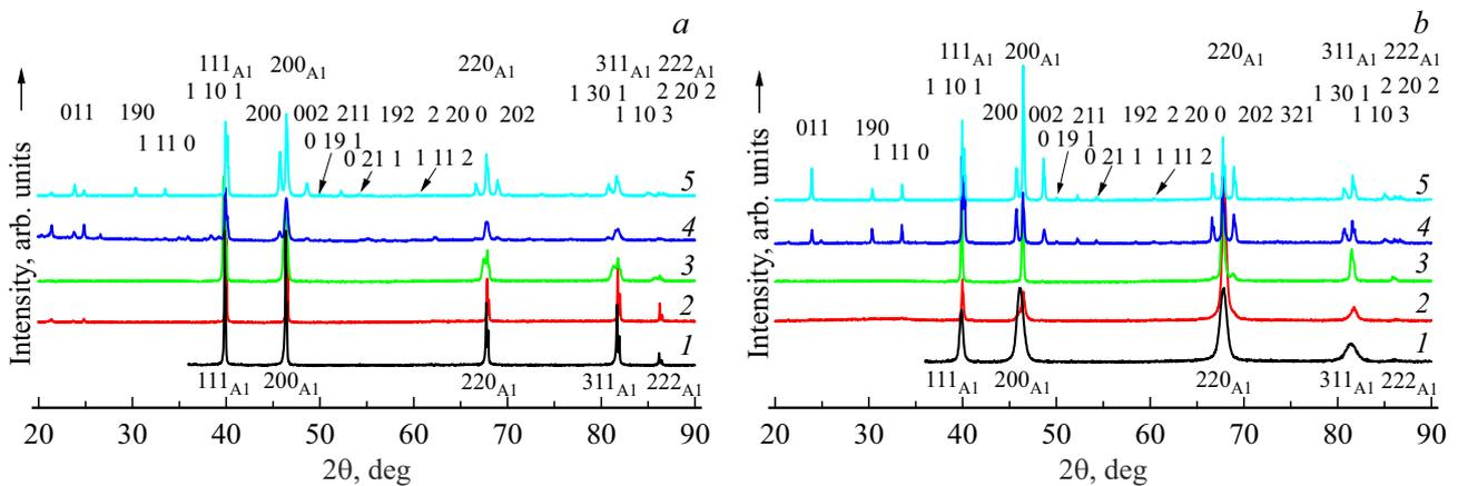
**Figure 5.** XRD results of samples of quenched (a) and deformed (b) alloy in initial state (I), after annealing for 1 (2), 24 (2), 168 (4) and 1440 h (3) at temperature of 375°C.
