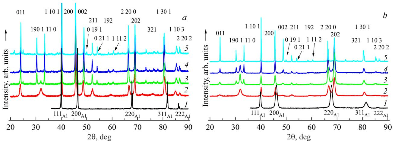
**Figure 4.** XRD results of samples of quenched (a) and deformed (b) alloy in initial state (I), after annealing for 1 (2), 24 (2), 168 (4) and 1440 h (3) at temperature of 325°C.
