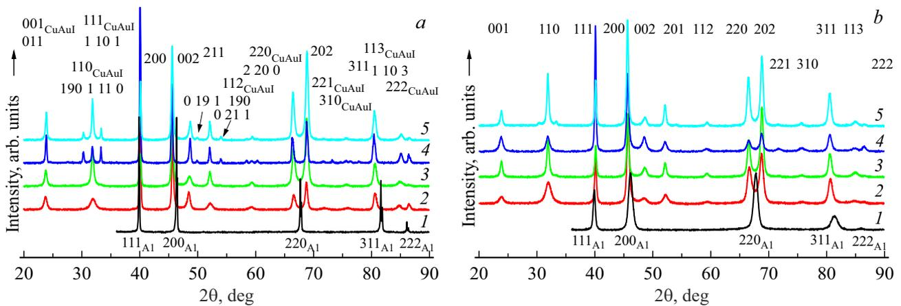
**Figure 3.** XRD results of samples of quenched (a) and deformed (b) alloy in initial state (I), after annealing for 1 (2), 24 (2), 168 (4) and 1440 h (3) at temperature of 300°C.
