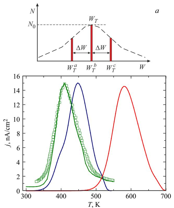
**Figure 4.** *a* — model when trap concentration is distributed as per Gaussian law depending on their energy, *b* — comparison of TSD experiment (*1* — squares) with calculation (*2, 3, 4* — solid lines) for Gaussian distribution of traps  $c = 1.15$  eV at depolarization voltage 4 V. Values of dispersion (distance between levels of traps  $\Delta W$ ) is: *2* — 0.01, *3* — 0.1, *4* — 0.5 eV.
