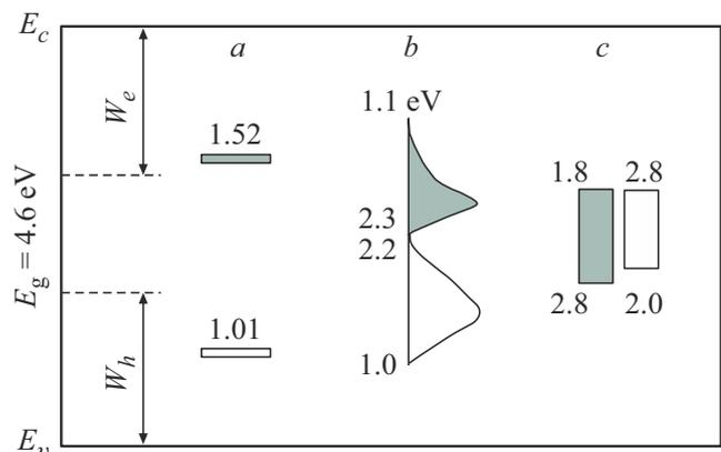
**Figure 1.** Energy spectrum of localized states for electrons and holes in amorphous  $\text{Si}_3\text{N}_4$  as per data from different papers. Numbers inside the Figure mark values of trap energy taken from papers: a — [19], b — [20], c — [21].
