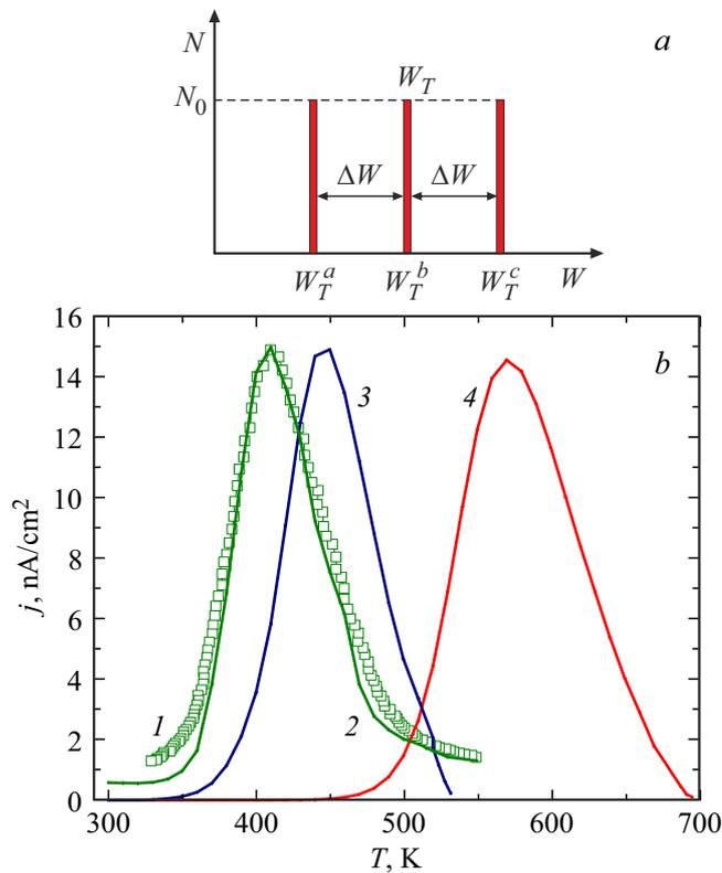
**Figure 3.** *a* — model of continuous spectrum of traps with three different energy levels and same concentration  $N_0$ ; *b* — comparison of TSD experiment (*1* — squares) with calculation (*2, 3, 4* — solid lines) for model of continuous spectrum of traps with  $W_T^b = 1.15$  eV at depolarization voltage 4 V. Values of dispersion (distance between levels of traps  $\Delta W$ ) is: *2* — 0.01, *3* — 0.1, *4* — 0.5 eV.
