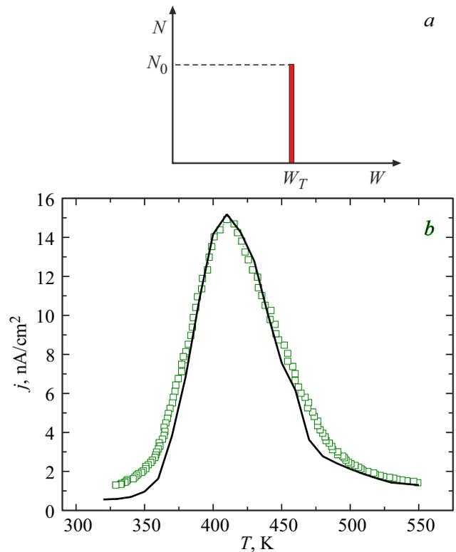
**Figure 2.** *a* — Model of discrete level of trap with energy  $W_T$  and concentration  $N_0$  in  $\text{Si}_3\text{N}_4$ , *b* — dependence of current on temperature at positive voltage 4 V on Al. Squares — experiment, dashed line — calculation for discrete level with energy  $W_T = 1.15$  eV.
