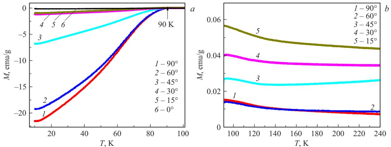
**Figure 1.** *a* — Temperature dependences of magnetization of an HTSC tape  $M(T)$  at  $H = 1$  kOe and different orientations of the magnetic field relative to the tape plane,  $T < 100$  K. *b* —  $M(T)$  plotted at  $T > 90$  K on an enlarged scale.
