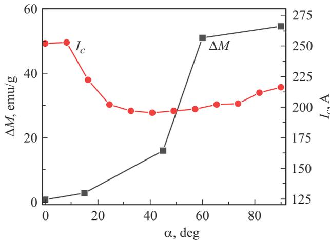
**Figure 3.** Dependences of magnetization loop height  $\Delta M$  ( $H = 0$ ) at  $T = 30$  K and critical tape current  $I_c$  at  $T = 77$  K and  $H = 500$  Oe on the angle of application of the external magnetic field.
