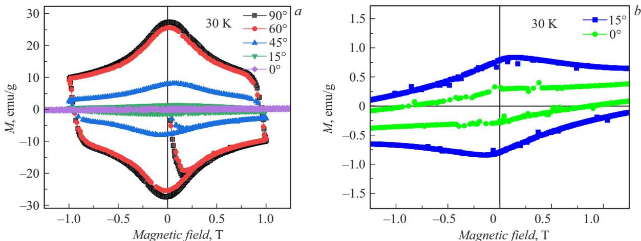
**Figure 2.** *a* — Dependence of tape magnetization on magnetic field  $M(H)$  at  $T = 30$  K and different angles between the tape plane and the magnetic field direction. *b* — Dependences  $M(H)$  plotted for angles of 0 and 15° on an enlarged scale.
