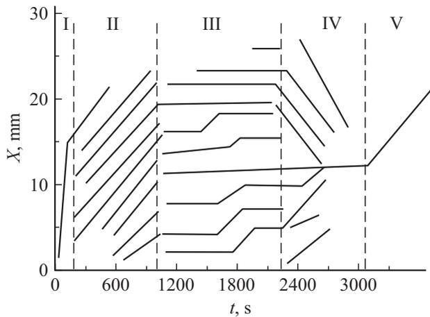
**Figure 1.** Stages of plastic flow under tension in a single crystal of the Fe–Cr–Ni alloy in the presence of atomic hydrogen (50 ppm). I — Lüders strain, II — stage of linear strain hardening, III — stage of parabolic strain hardening, IV — collapse of the autowave function (pre-fracture), and V — necking.
