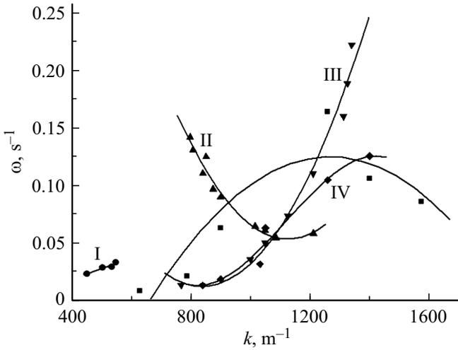
**Figure 2.** Dispersion curves for different stages. Squares — easy slip [2], circles — Lüders strain (I), triangles — linear strain hardening (II), inverted triangles — parabolic strain hardening (III), and diamonds — pre-fracture (IV).
