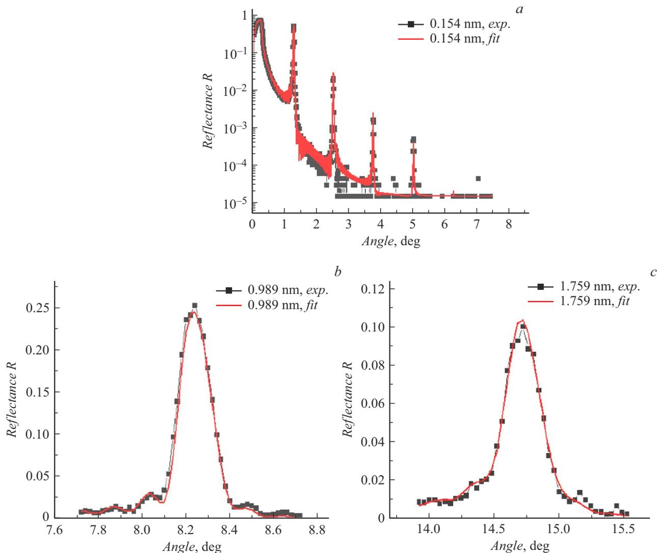
**Figure 2.** Dependences of the experimentally measured reflectance on the grazing angle of incidence and the results of fitting for wavelengths  $\lambda = 0.154$  (a), 0.989 (b), and 1.759 nm (c).
