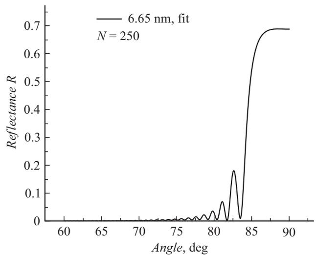
**Figure 3.** Theoretical dependence of reflectance on the grazing angle of incidence at wavelength  $\lambda = 6.65$  nm for a multilayer Ru/C/B mirror calculated with account for the obtained structural parameters.
