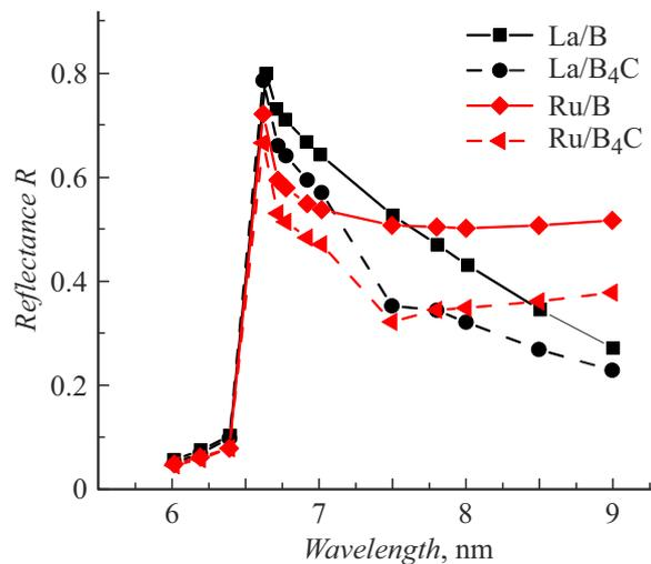
**Figure 1.** Reflectance dependences for ideal La/B, La/B<sub>4</sub>C, Ru/B, and Ru/B<sub>4</sub>C structures within the range of 6–9 nm at a grazing angle of incidence of  $90^\circ$ . Optical constants from the CXRO database ([https://henke.lbl.gov/optical\\_constants/](https://henke.lbl.gov/optical_constants/)) were used in calculations.
