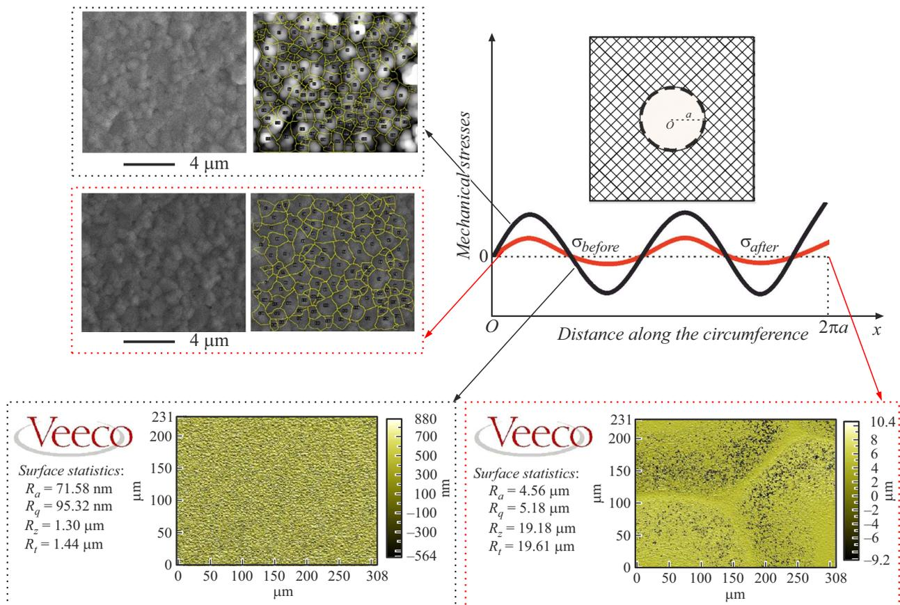
**Figure 3.** Explanations for the effect of variations in mechanical properties: schematic pattern of the mechanical stress distribution over the membrane before and after heat treatment, results of the grain size analysis in the ImageJ code, measurements of surface roughness before and after heat treatment.
