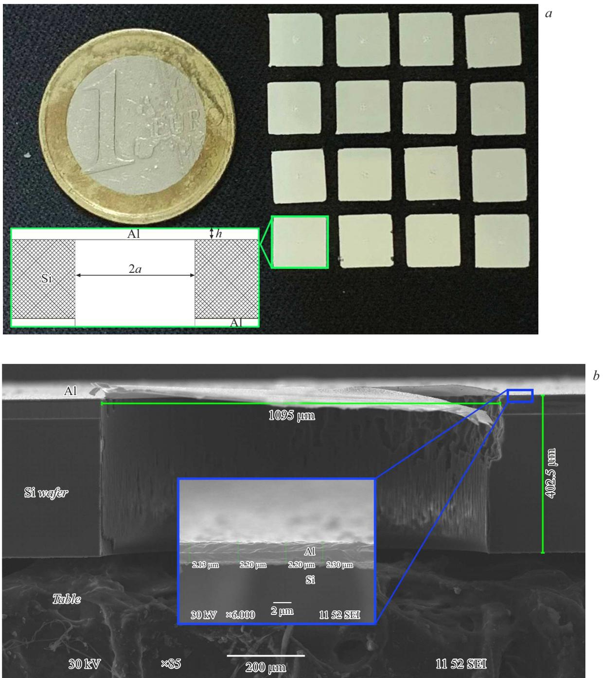
**Figure 1.** Structures to be studied. *a* — structure schematic diagram (side view); *b* — SEM image of the aluminum film.
