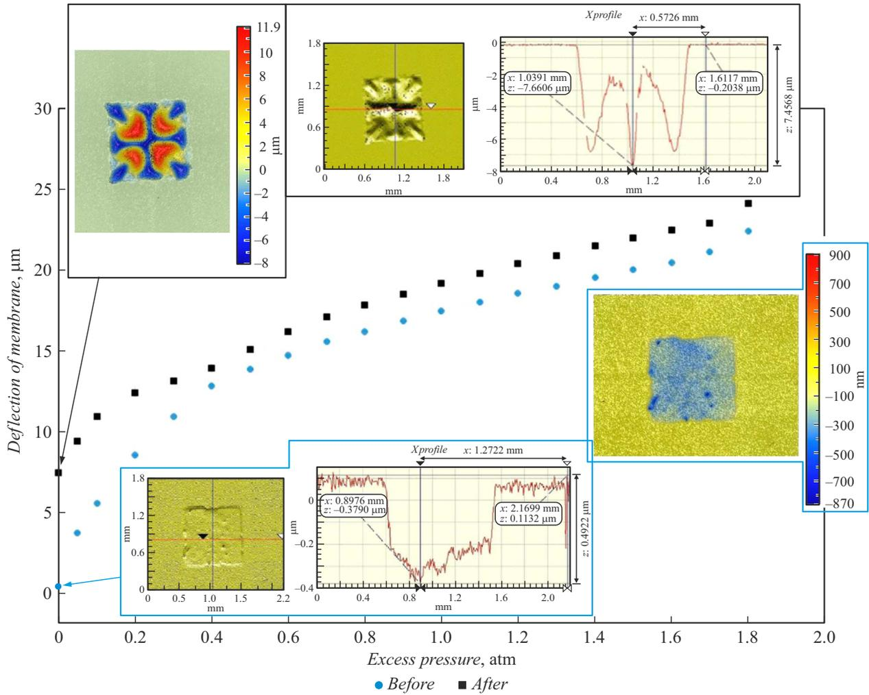
Figure 2. Square membrane deflection versus excess pressure before and after heat treatment.
