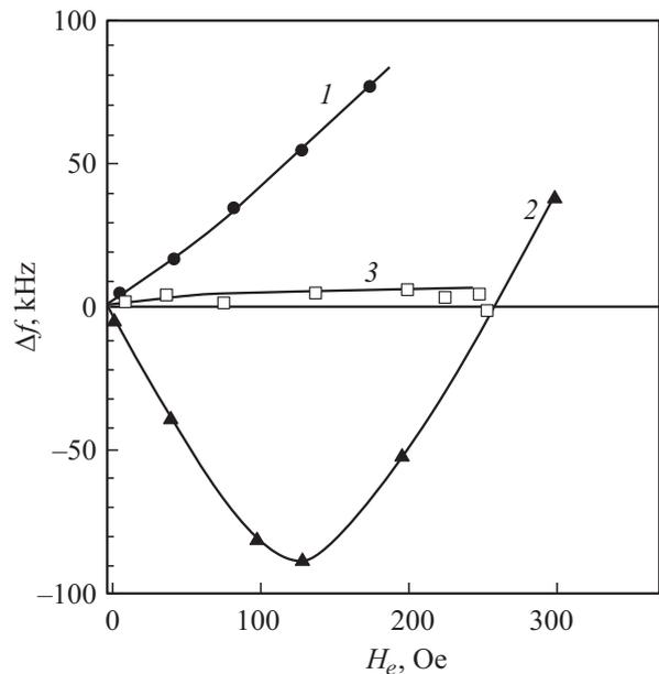
**Figure 1.** Resonant frequency of the LC generator with a cobalt-composite sample in its resonant circuit versus magnetic field  $H_e$ . 1 — along the sample magnetization, 2 — in the opposite direction, 3 — perpendicular to magnetization.
