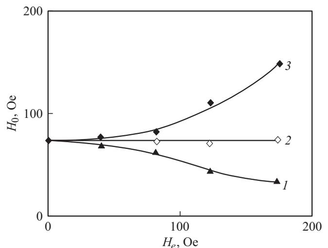
**Figure 3.** Pinning force  $H_0$  versus external field  $H_e$  for three external field directions: opposite to (1), across (2) and along (3) the sample magnetization.  $\tau_m = 1 \mu\text{s}$ .
