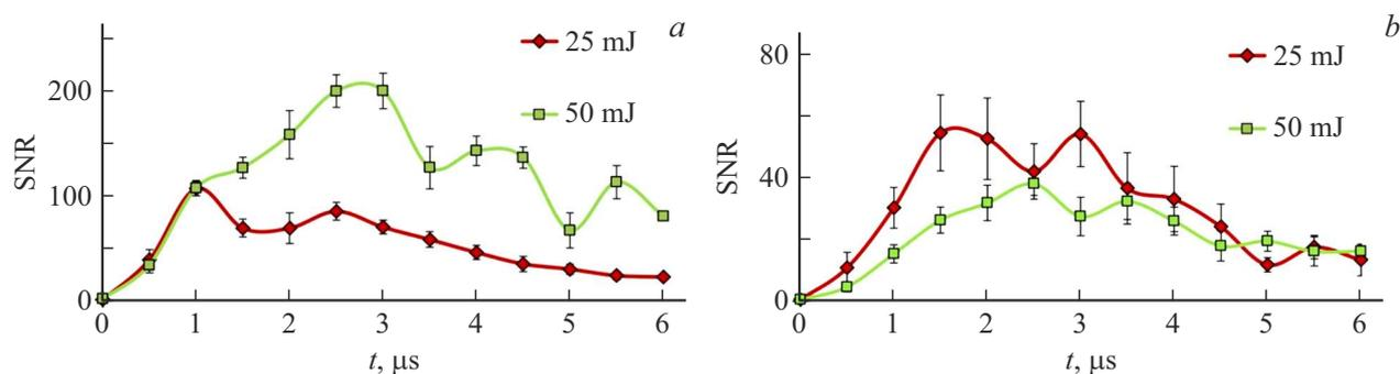
**Figure 3.** SNR versus the detection delay at the exciting pulse energies of 25 and 50 mJ. *a* — Ba,  $\text{NA} = 0.02$ ; *b* — Al,  $\text{NA} = 0.04$ .
