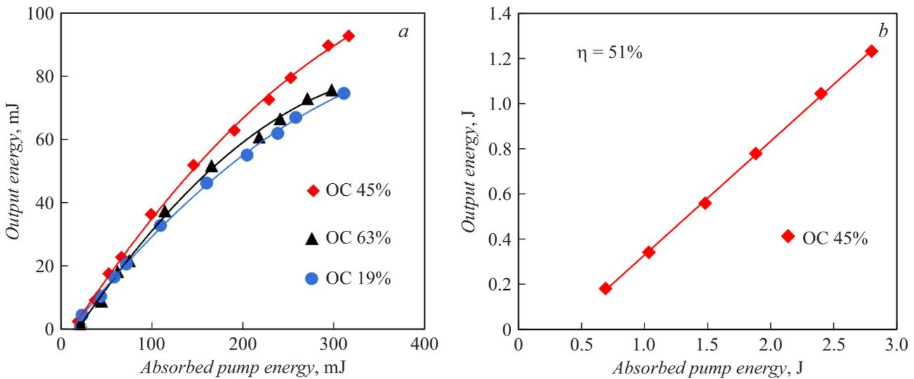
**Figure 2.** Dependences of the  $\text{Cr}^{2+}:\text{CdSe}$  laser output energy on absorbed pump energy, which were obtained using different outcoupling mirrors at the pump spot diameters of 1.4 (a) and 4.7 mm (b).
