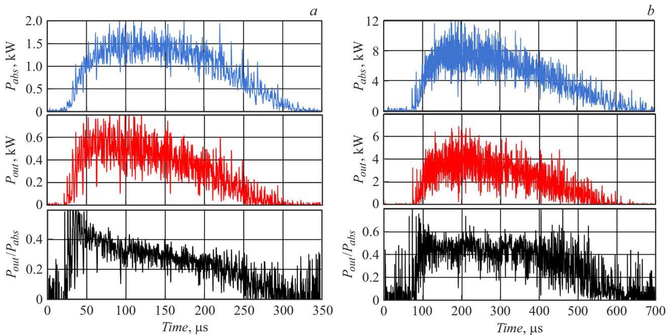
**Figure 3.** Shapes of the pump pulse (top oscillogram) and lasing pulse (middle oscillogram), and the lasing power to pump power ratio (bottom oscillogram). *a* — pump beam diameter is 1.4 mm, absorbed pump energy is 300 mJ; *b* — pump beam diameter is 4.7 mm, absorbed pump energy is 2.6 J.
