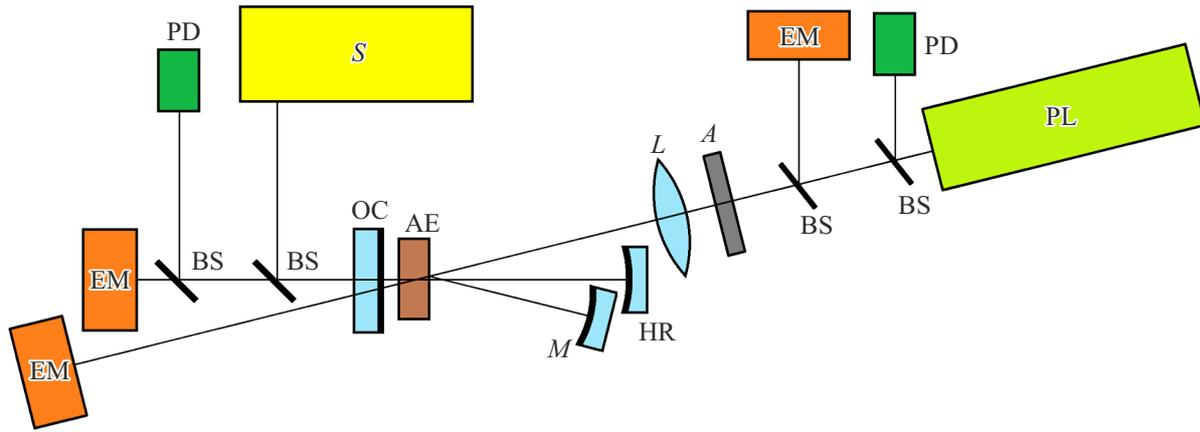
**Figure 1.** Experimental details. PL — pump laser, BS — beam splitter, PD — photodiode, EM — energy meter,  $L$  — focusing lens,  $A$  — beam attenuator, HR and OC — totally reflecting and outcoupling mirrors of the  $\text{Cr}^{2+}:\text{CdSe}$  laser cavity, AE —  $\text{Cr}^{2+}:\text{CdSe}$  crystal,  $M$  — spherical Al mirror,  $S$  — diffraction-grating spectrograph.
