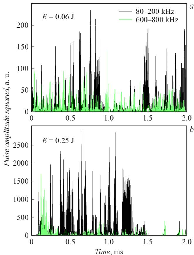
**Figure 3.** Time scans of AE amplitudes in the ranges of 80–200 and 600–800 kHz, recorded in the case of damages produced by impacts with energies of 0.06 (a) and 0.25 J (b) at the temperature of 110°C. The colored figure is given in the electronic version of the paper.
