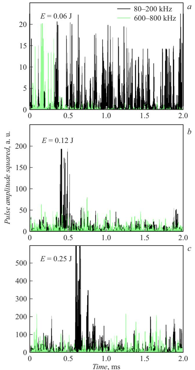
**Figure 1.** Time scans of AE amplitudes in the ranges of 80–200 and 600–800 kHz, which were recorded in the case of damages by impacts with energies of 0.06 (*a*), 0.12 (*b*) and 0.25 J (*c*) produced at the sample temperature of 20°C. The colored figure is given in the electronic version of the paper.
