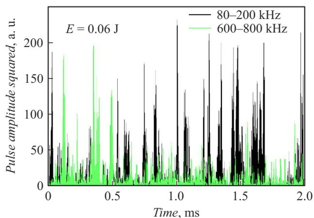
**Figure 2.** Time scans of AE amplitudes in the 80–200 and 600–800 kHz ranges recorded for the case of damage by the impact 0.06 J in energy at the temperature of 80°C. The colored figure is given in the electronic version of the paper.
