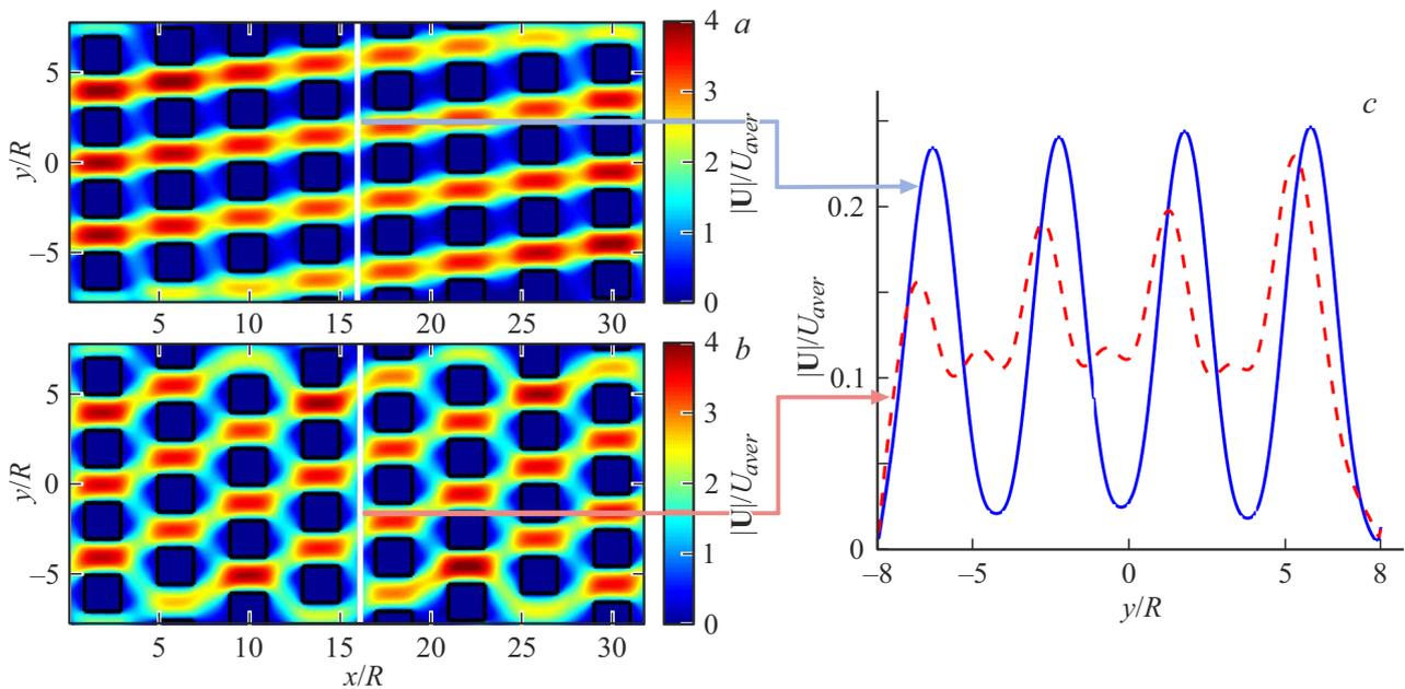
**Figure 2.** Distribution of velocity modulus  $|U|/U_{aver}$  at row displacement  $d = 5$  (a) and  $15 \mu\text{m}$  (b). c — Velocity profile between the rows.
