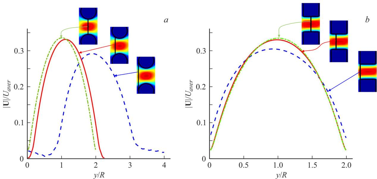
**Figure 3.**  $|U|/U_{aver}$  velocity profiles at different points between two adjacent round (a) and square (b) pillars or posts.
