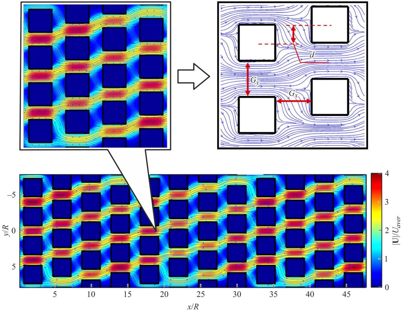
**Figure 1.** Distribution of velocity modulus  $|\mathbf{U}|/U_{aver}$  and streamlines in a microchannel with DLD at  $d = 10 \mu\text{m}$ .
