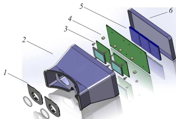
**Figure 1.** Testing device. 1 — Eyepiece, 2 — case, 3 — display, 4 — driver, 5 — main board with a radio module, and 6 — back cover.
