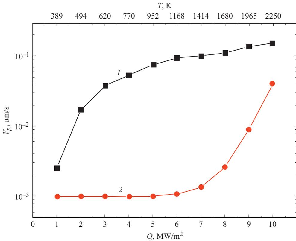
**Figure 1.** Dependences of rate  $V_p$  of ion (1) and thermal (2) sputtering of reactor graphite on power input  $Q$  into the discharge and the corresponding temperature  $T$  of the processed graphite surface.
