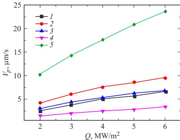
**Figure 2.** Dependences of rate  $V_p$  of ion sputtering of radioactive deposits (1 — NiCrFeO<sub>4</sub>, 2 — NiFe<sub>2</sub>O<sub>4</sub>, 3 — Fe<sub>2</sub>O<sub>3</sub>, 4 — TiO<sub>2</sub>, 5 — U<sub>3</sub>O<sub>8</sub>) on the internal circuit equipment of NPPs on power input  $Q$  into the discharge.
