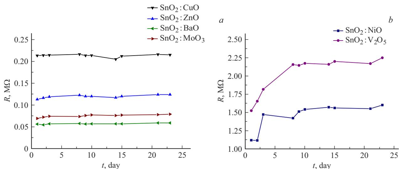
**Figure 1.** Stability of the electrophysical characteristics of sensors in laboratory air.
