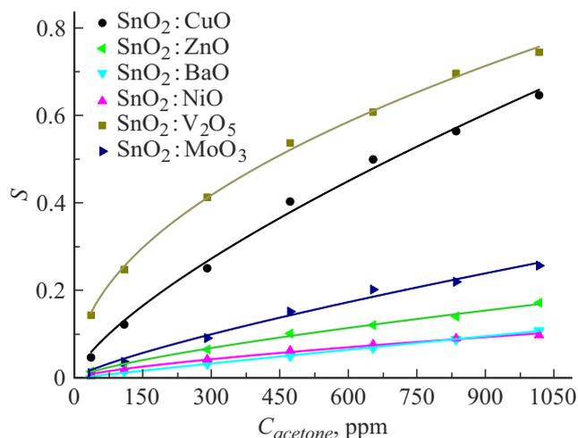
**Figure 2.** Concentration dependences of the sensitivity of sensors to acetone.
